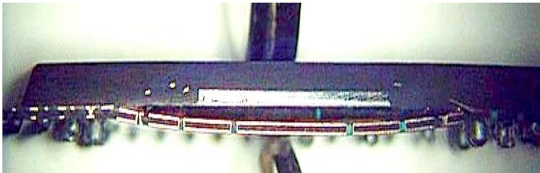
Figure 34. BGA Cross Section Exhibiting Moisture Damage (Popcorning)
