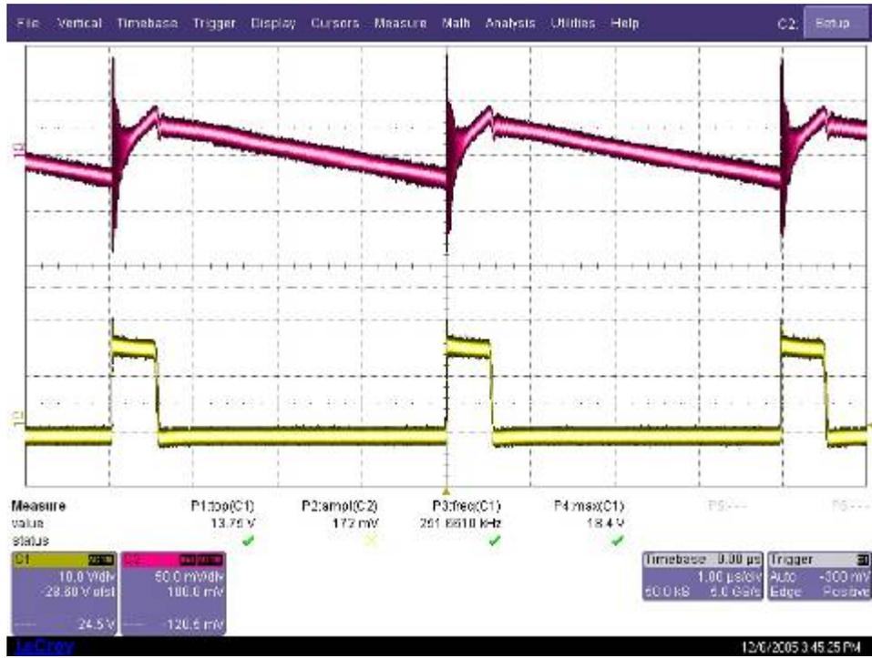
Figure 16.  $V_{in} = 18\text{ V}$ ,  $V_{out} = 1.8\text{ V}$ ,  $I_{out} = 1.5\text{ A}$ ,  $C1 = V_{out}$ ,  $C2 = V_{SW}$
