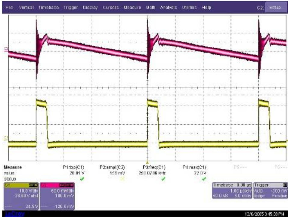
Figure 17.  $V_{in} = 24\text{ V}$ ,  $V_{out} = 1.8\text{ V}$ ,  $I_{out} = 1.5\text{ A}$ ,  $C1 = V_{out}$ ,  $C2 = V_{SW}$
