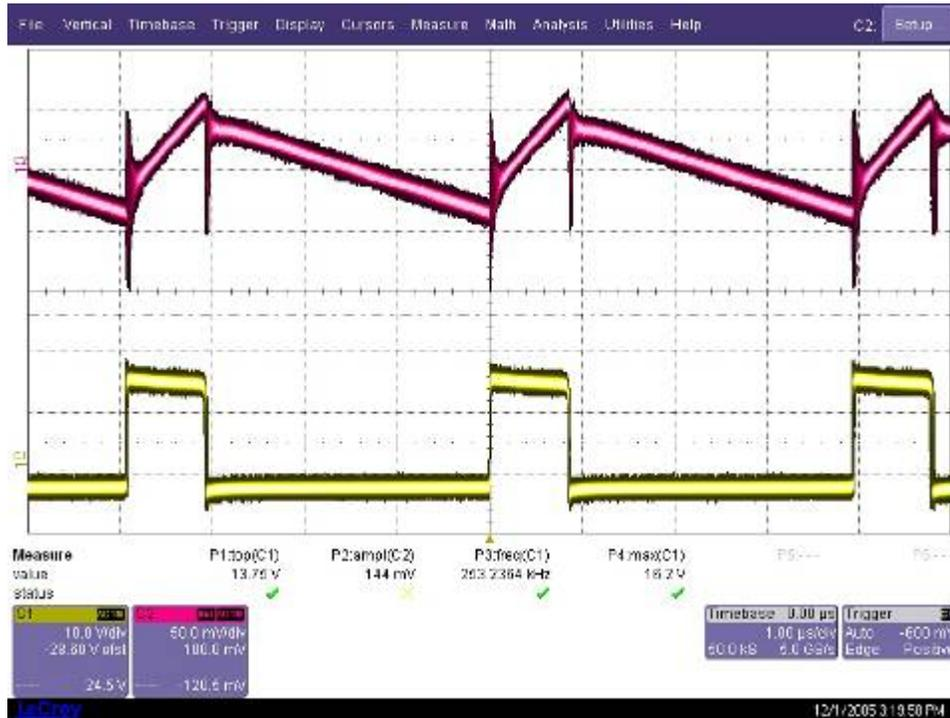
Figure 11. Vin = 18 V, Vout = 3.3 V, Iout = 1.5 A, C1 = Vout, C2 = VSW
