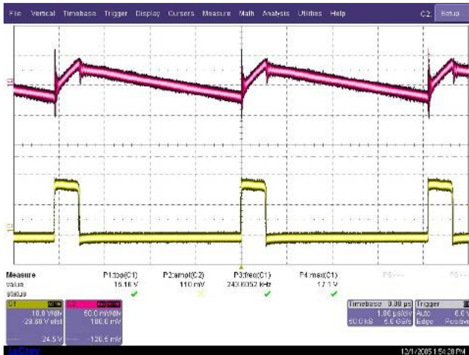
Figure 8.  $V_{in} = 18\text{ V}$ ,  $V_{out} = 1.8\text{ V}$ ,  $I_{out} = 1.5\text{ A}$ ,  $C_1 = V_{out}$ ,  $C_2 = V_{SW}$
