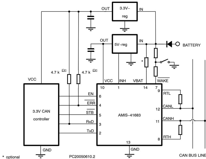
Figure 4. Dual V<sub>CC</sub> Topology for 3.3 V Microcontroller
