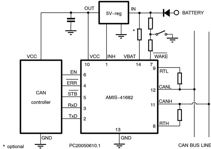
Figure 3. Single V<sub>CC</sub> Topology for 5 V Microcontroller
