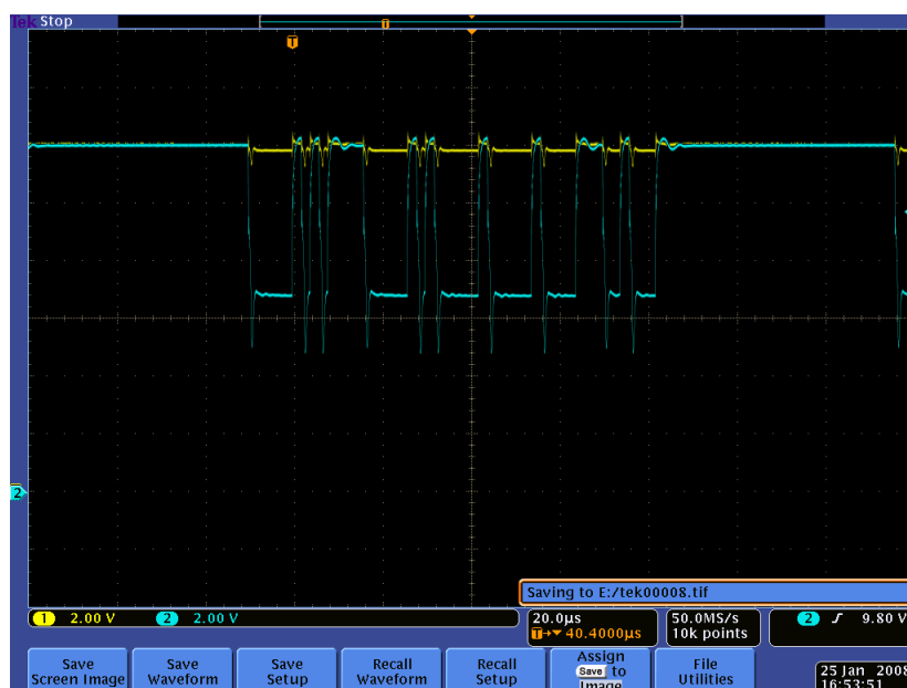
Figure 8. Data Frame Periodically Sent by the HS-CAN Node when CAHL is Shorted to 12 V – Yellow Trace = CANH; Blue Trace = CANL
