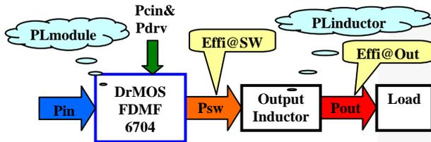
Figure 2. Ploss Diagram of FDMF6704 Eval Board
