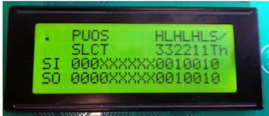
b. Remove the ULD 1 jumper. Confirm the display and the motor is off.
