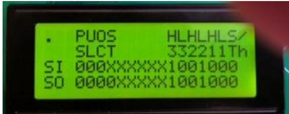
j. Remove the UVLO jumper. Confirm the display and the motor is off.
