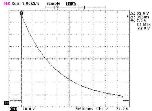
**Figure 9. Load Dump Transient Waveform (60 V, 350 ms).**
