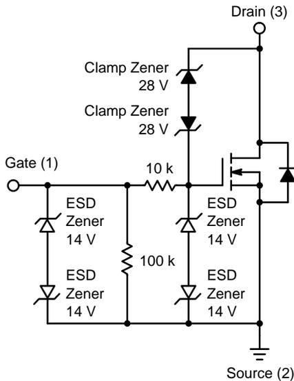
**Figure 5. Automotive Relay Driver Description (NUD3124 Device)**
