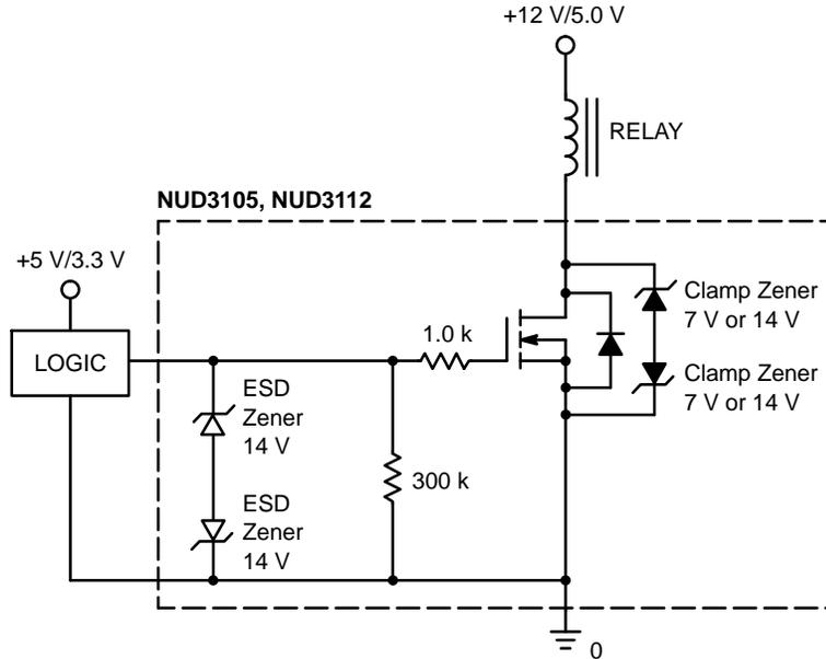
**Figure 3. Typical Connection Diagram
