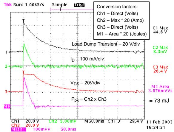
Figure 10. Waveforms Generated Across the NUD3124 Device During a Load Dump Transient
