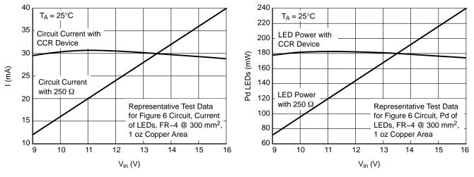
Figure 2. Series Circuit Current
