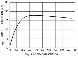
Figure 10. CCR–IV Characteristics @ 255C
