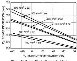
Figure 11. Power Dissipation vs. Ambient Temperature @ T<sub>J</sub> = 150°C for Variable Copper Heat Spreader
