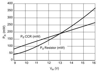
Figure 9. CCR P<sub>d</sub> vs. Resistor Pd
