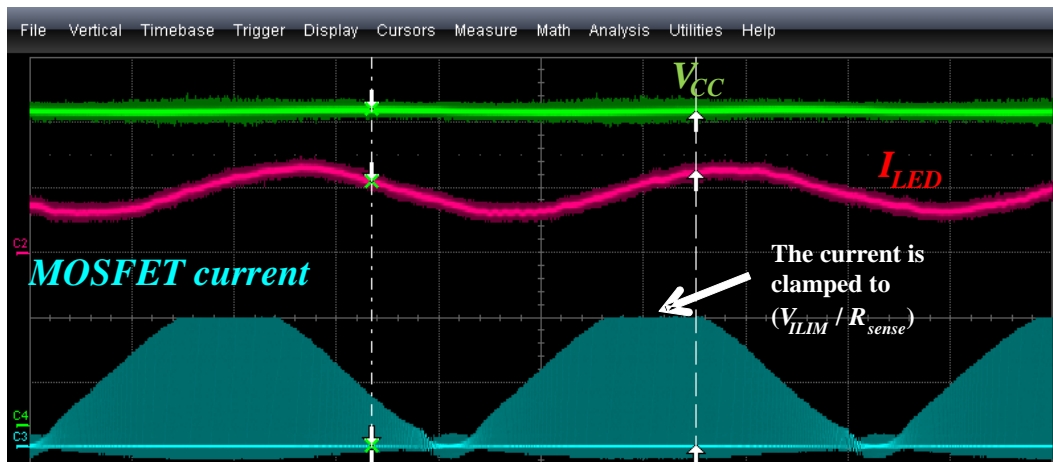
Figure 2. Current Over-Current Limitation ( V_{ILIM} is the Over-Current Threshold, R_{SENSE} the Current Sense Resistor)
