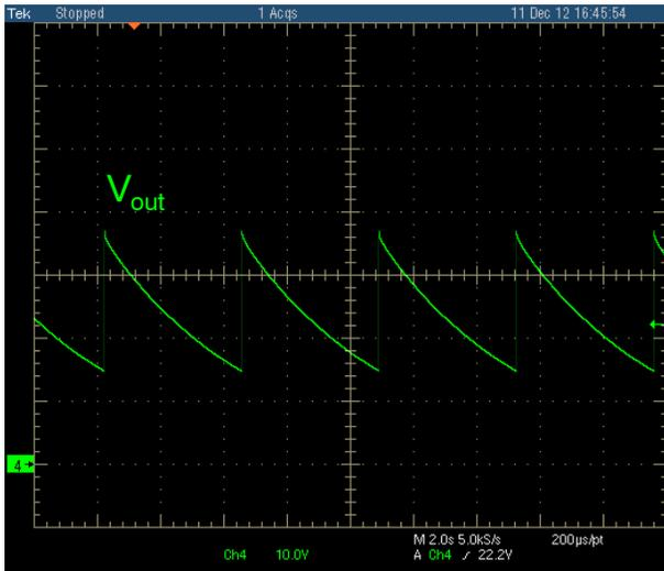
Figure 14. Output Voltage Variation with No Output Load
