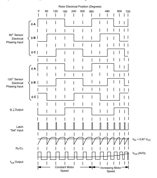
Figure 3. Timing Diagram of a Typical Three Phase, SIx Step Motor Application
