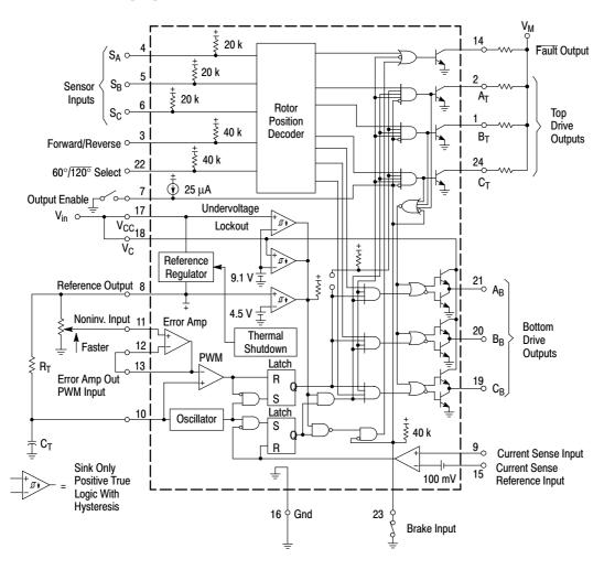
Figure 1. MC33035 Representative Block Diagram
