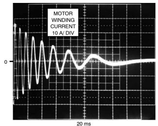
Figure 9. Application of Brake Signal May Produce Large Fault Currents
