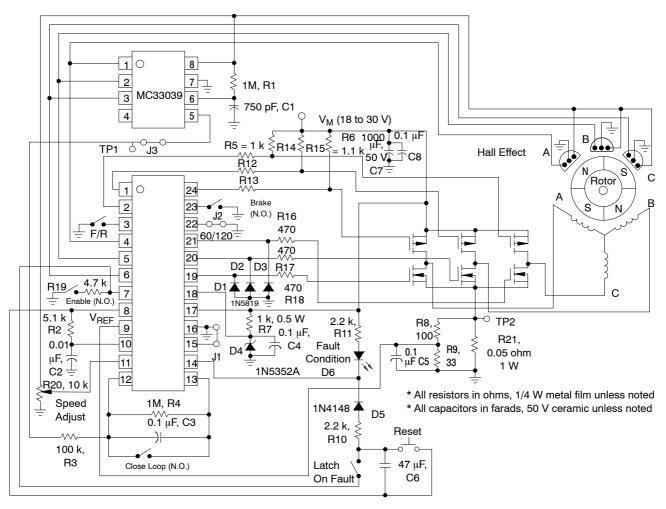
Figure 6. Typical 24 V Brushless Motor Drive (with 120 Degree Sensor Phasing)
