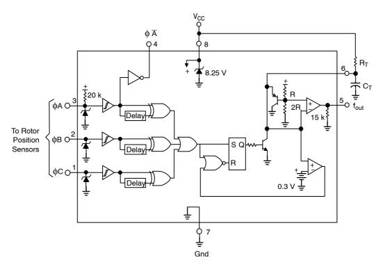
Figure 4. Representative Block Diagram of MC33039
