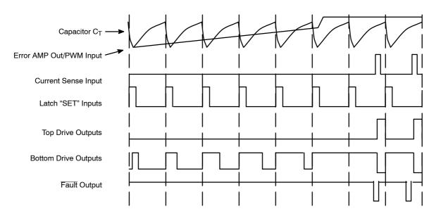
Figure 2. The MC33035's Pulse-Width Modulator Timing Diagram
