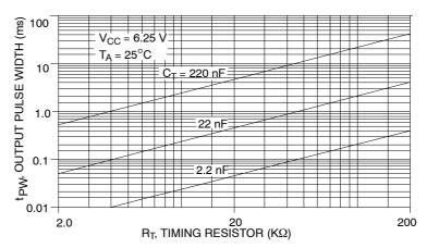
Figure 5. fout Pulse Width versus Timing Resistor
