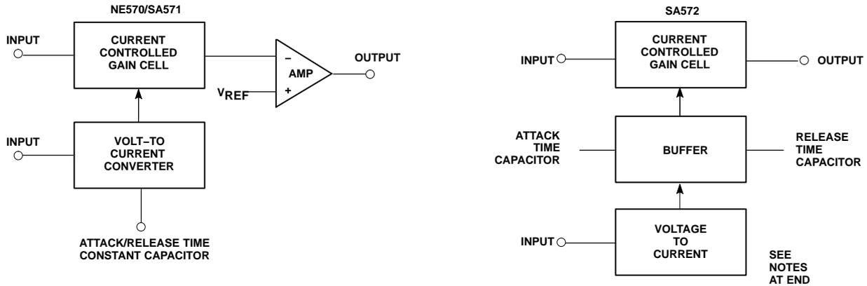
Figure 5. Block Diagrams
