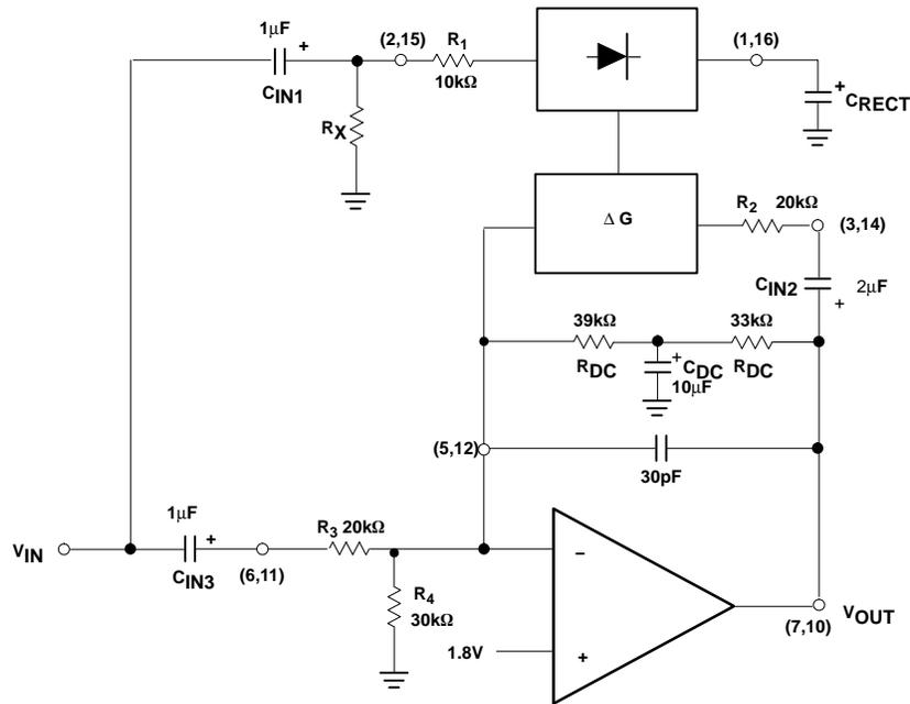
**Figure 10. Automatic Level Control
