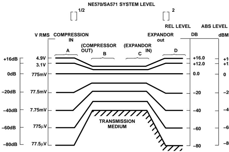
Figure 11. System Levels of a Complete Companding System
