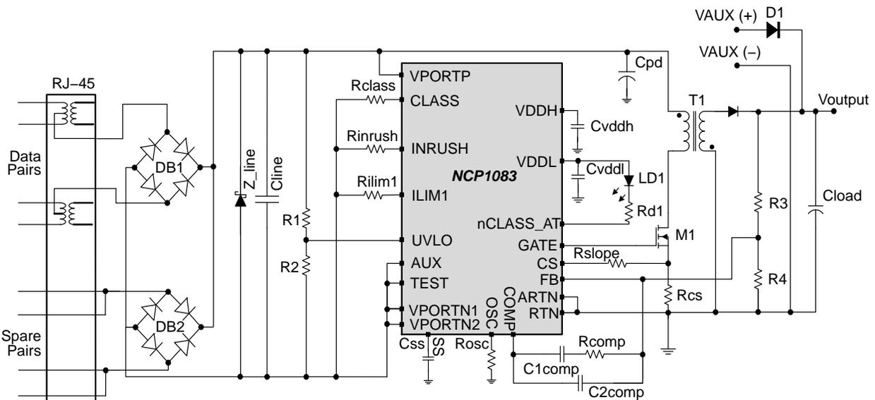
Figure 3. Direct Auxiliary Supply Configuration
