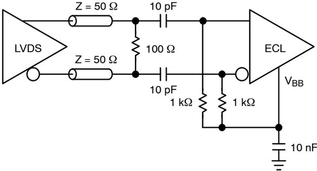
**Figure 3. Capacitive Coupling LVDS to ECL Using  $V_{BB}$**
