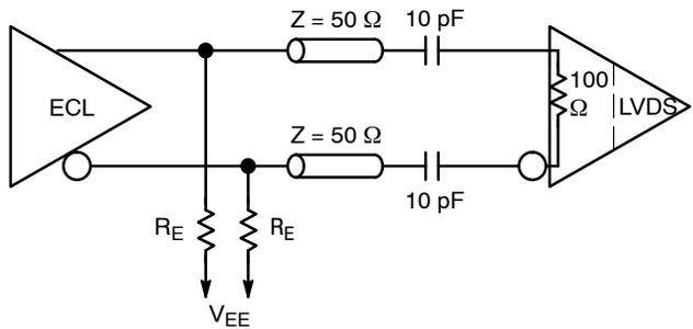
**Figure 5. Capacitive Coupling ECL to LVDS**
