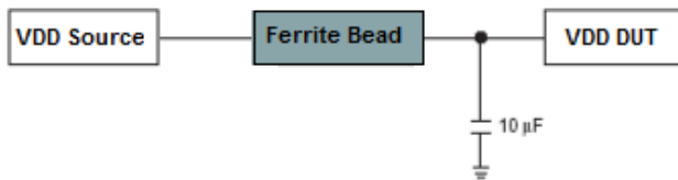
Figure 9. Power Supply Noise Filtering Example
