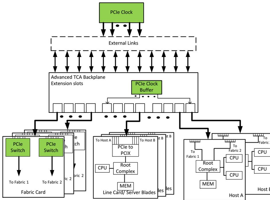
Figure 7. Typical Clock Tree in Embedded Applications
