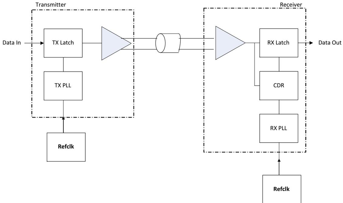
Figure 3. Separate Reference Clock with Independent Spread Architecture
