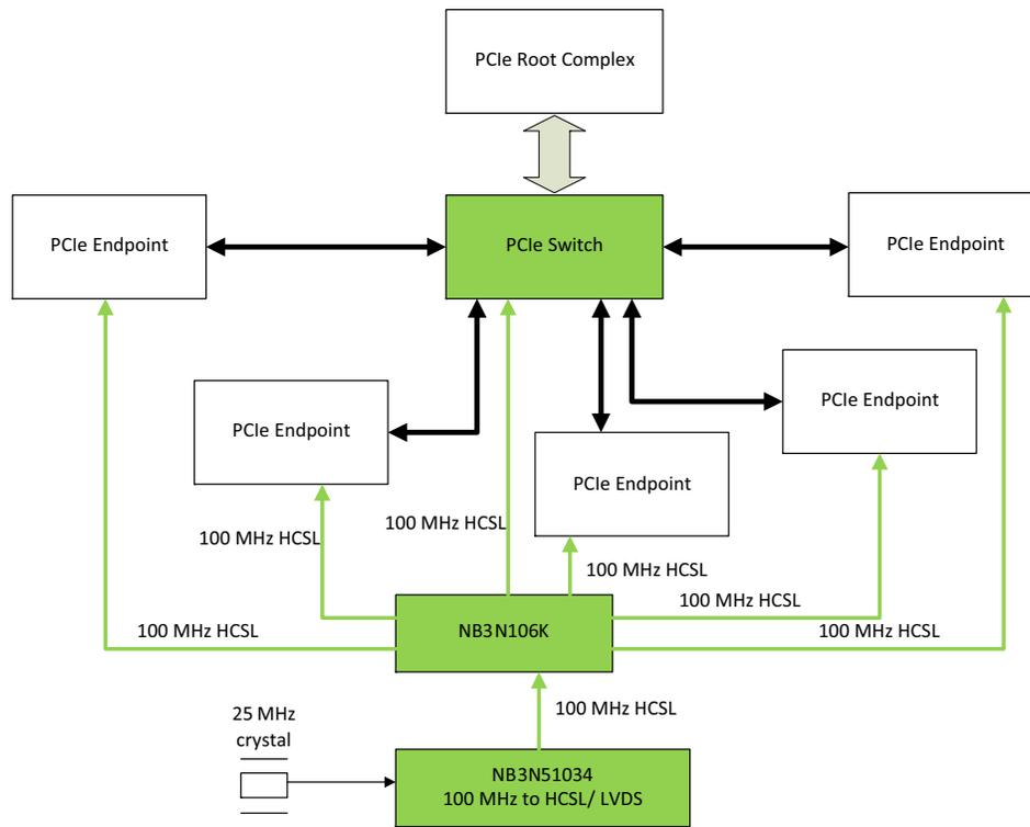
Figure 6. Typical Clock Tree in Computation Applications
