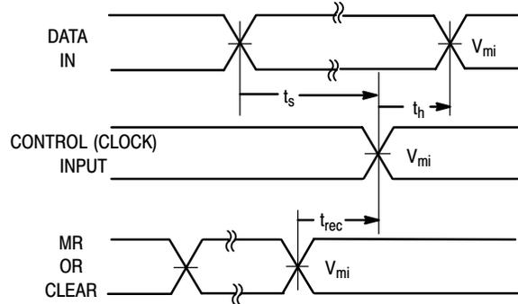
Figure 3-7. Setup Time, Hold Time and Recovery Time
