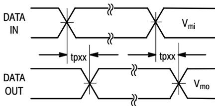
Figure 3-5. Waveform for Inverting and Non-Inverting Functions
