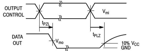
Figure 3-9. 3-State Output Low Enable and Disable Times
