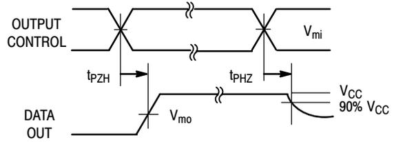
Figure 3-8. 3-State Output High Enable and Disable Times
