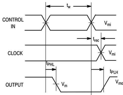
Figure 3-6. Propagational Delay, Pulse Width and  $t_{rec}$  Waveforms
