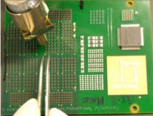
**Figure 4. Removal of Device Using Hot Air Source**
