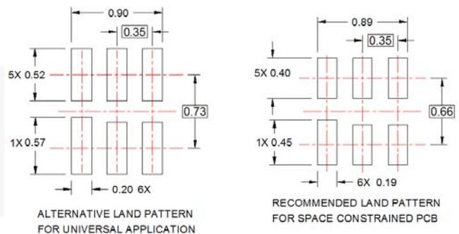
Figure 1. Schematic of Dimensions of Pad Designs
