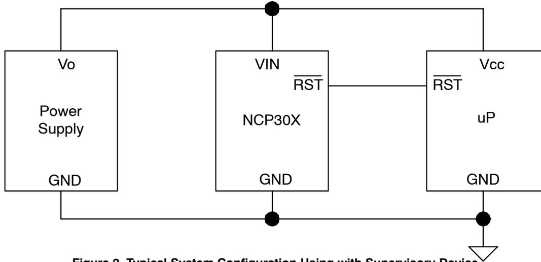
**Figure 2. Typical System Configuration Using with Supervisory Device**
