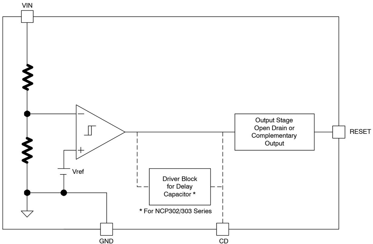
**Figure 1. General Block Diagram of NCP30X Family Series**
