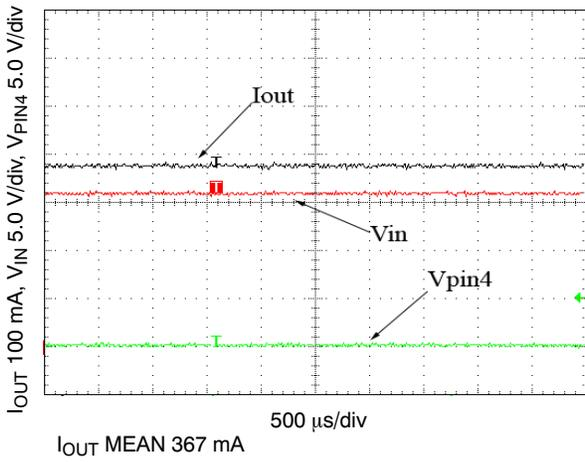
Figure 5. Circuit Behavior at 100% Duty Cycle
