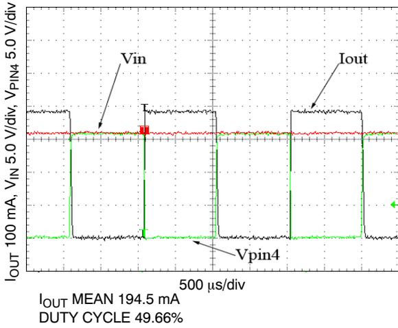
Figure 3. Circuit Behavior at ~50% Duty Cycle
