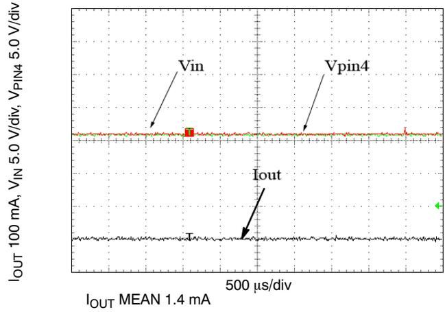
Figure 4. Circuit Behavior at 0% Duty Cycle
