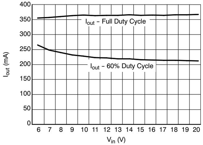
Figure 6. Output Current Regulation at 100% and 60% Duty Cycles
