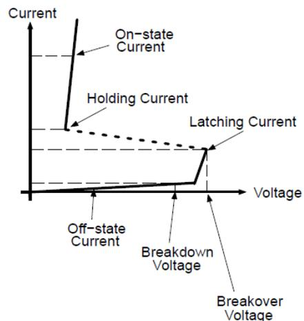
Figure 3. An example of I-V characteristics for an LED shunt.
