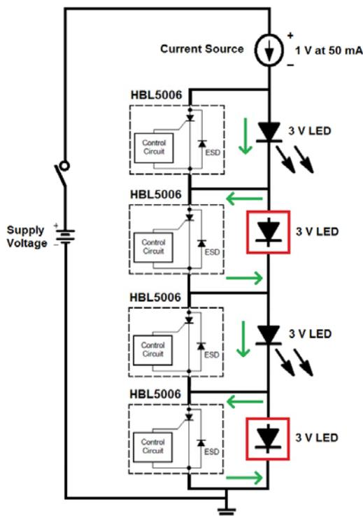
Figure 6. Adequate supply voltage must be provided for cases in which multiple LEDs have failed.
