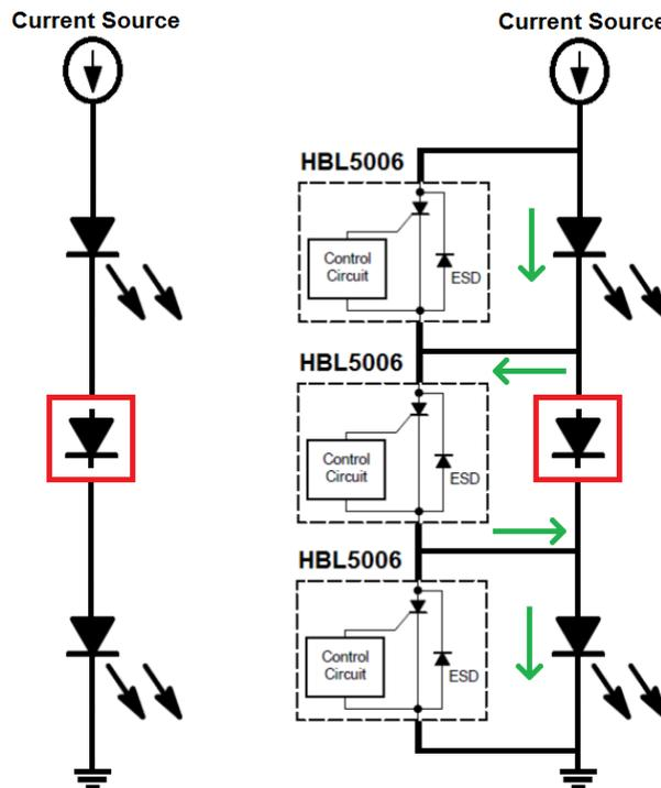
Figure 1. After an LED open circuit failure the entire string goes dark unless LED shunts are used.
