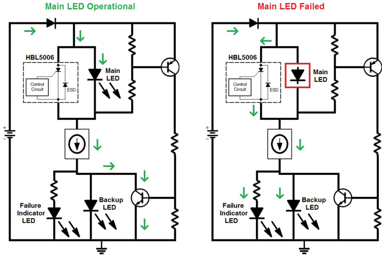
Figure 2. Failure detector circuit for critical lighting applications with backup LED and failure indicator LED. See Design Note DN05066 for more details.
