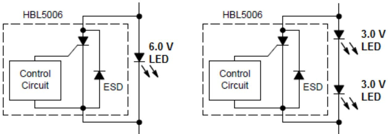
Figure 4. Examples of acceptable configurations for HBL5006. The forward voltage of the LEDs does not exceed the minimum breakdown voltage of the HBL5006 (6.2 V).
