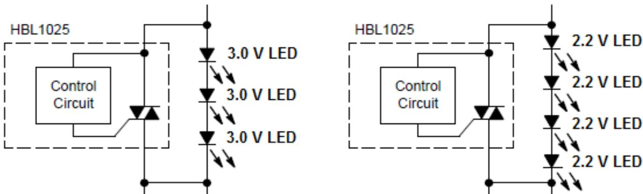
Figure 5. One HBL1025 can cover LED strings with forward voltages up to 11.5 V
