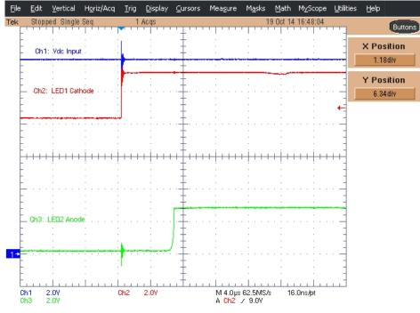
Figure 3: LED1 short circuit failure. LED2 turns on about 7 µs after LED1 fails.
