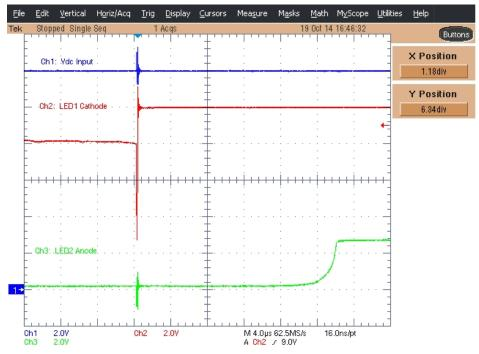
Figure 2: LED1 open circuit failure. LED2 turns on about 20 µs after LED1 fails.
