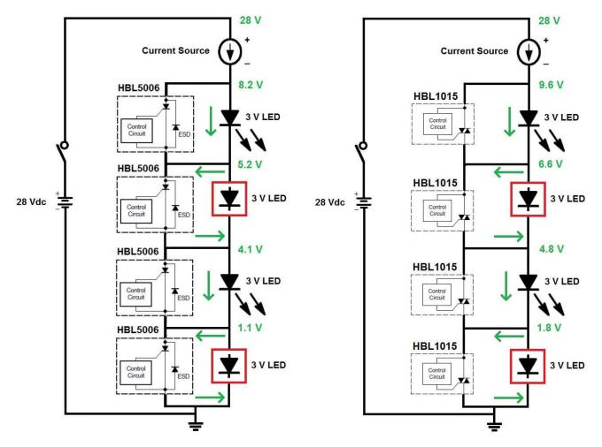
Figure 7. The HBL1015 has a higher on-state voltage. Therefore the voltage over the current source is not as high as it is in the HBL5006 case.
