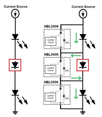
Figure 1. After an LED open circuit failure the entire string goes dark unless LED shunts are used.
