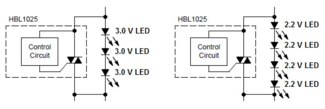
Figure 5. One HBL1025 can cover LED strings with forward voltages up to 11.5 V
