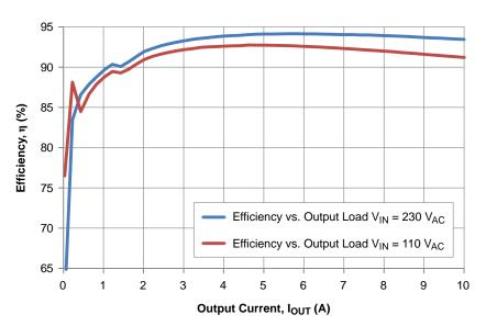
Figure 19. Board Efficiency – Including PFC Stage
