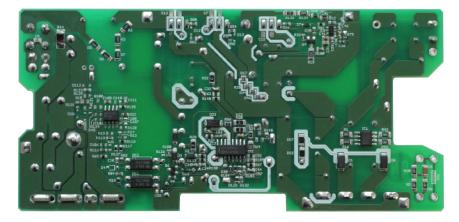
Figure 10. Main Board Photo – Bottom Side
