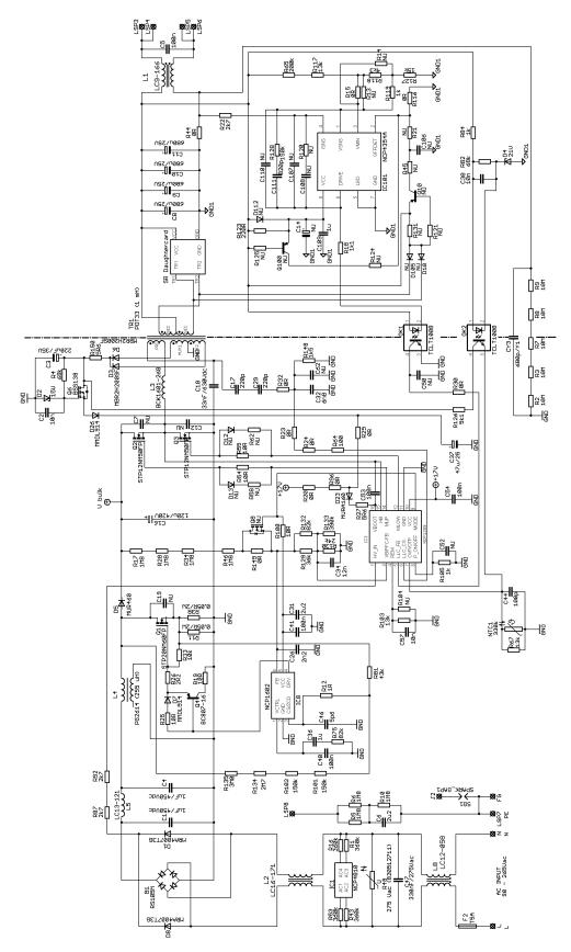
Figure 1. Laptop Adapter Demo-board – Main Board Schematic
