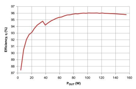
Figure 20. Board Power Stage with SR Efficiency  $V_{\text{IN}}$  = 385  $V_{\text{DC}}$
