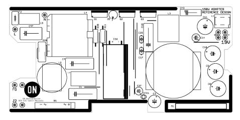
Figure 4. Main Board Top Side Components
