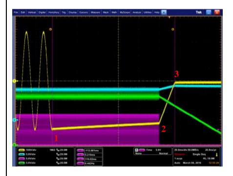
X2 Discharge at 265 VAC Ch. 1 (Yellow): VAC Input Ch. 2 (Blue): V<sub>cc</sub> Ch. 3 (Purple): DRV Ch. 4 (Green): V<sub>OUT</sub>
