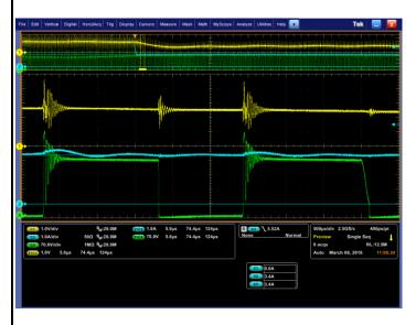
The NCP1341 features a power excursion mode which seamlessly transitions the system into a continuous conduction mode operation to allow for increased power delivery during load transients. PEM enables the system to deliver up to 2 times the nominal load.
