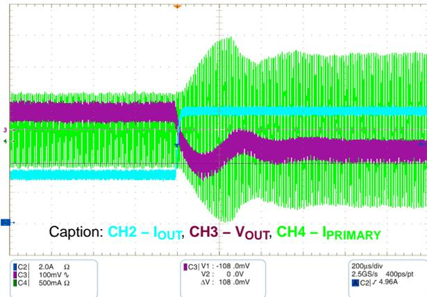
Figure 17. Transition Response – Load Step from 3 to 7 A
