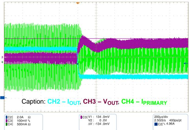
Figure 18. Transition Response – Load Step from 7 to 3 A
