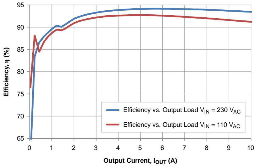
Figure 19. Board Efficiency – Including PFC Stage
