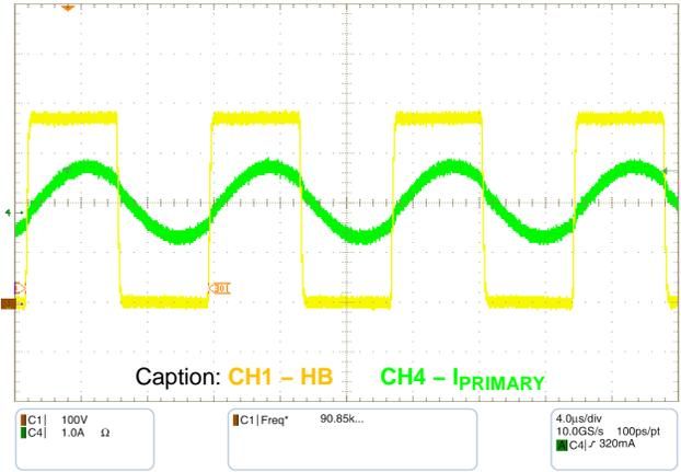
Figure 14. Steady Stage – I<sub>LOAD</sub> = 4 A
