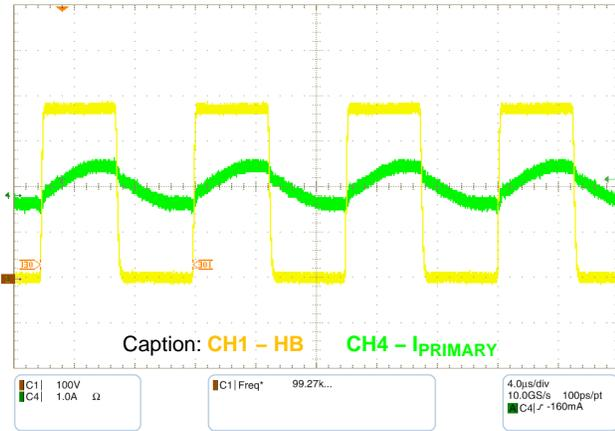
Figure 13. Steady Stage – I<sub>LOAD</sub> = 2 A
