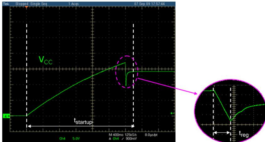
Figure 12.  $V_{CC}$  Waveform during Startup
