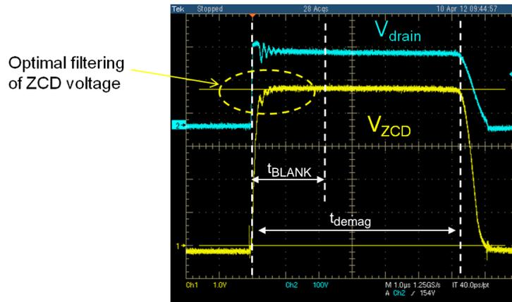
Figure 6. Optimal Filtering of ZCD Pin Voltage
