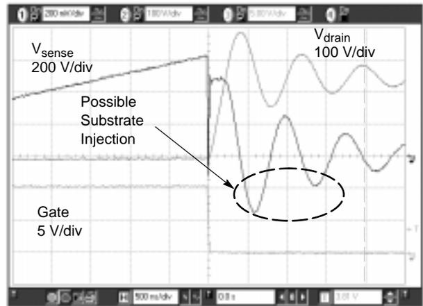
**Figure 11d.** As predicted by the calculations, the turn-off time is extremely fast and does not engender losses. The switch is immediately closed and the current is capacitive. This plot can be compared to Figure 10c.
