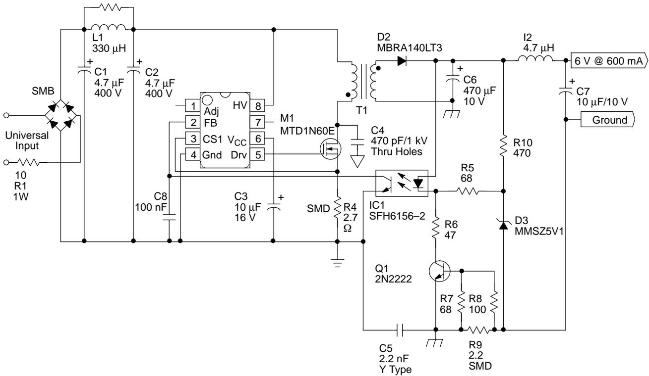
Figure 12e. The Complete Battery Charger Demonstration Board
