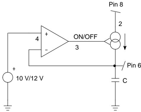
**Figure 1a. Internal Implementation of the Dynamic Self-Supply**
