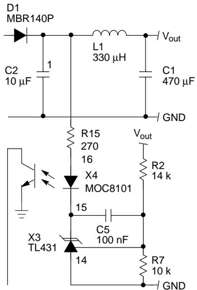
Figure 13. A Precise Regulation Option using a TL431 Reference Voltage
