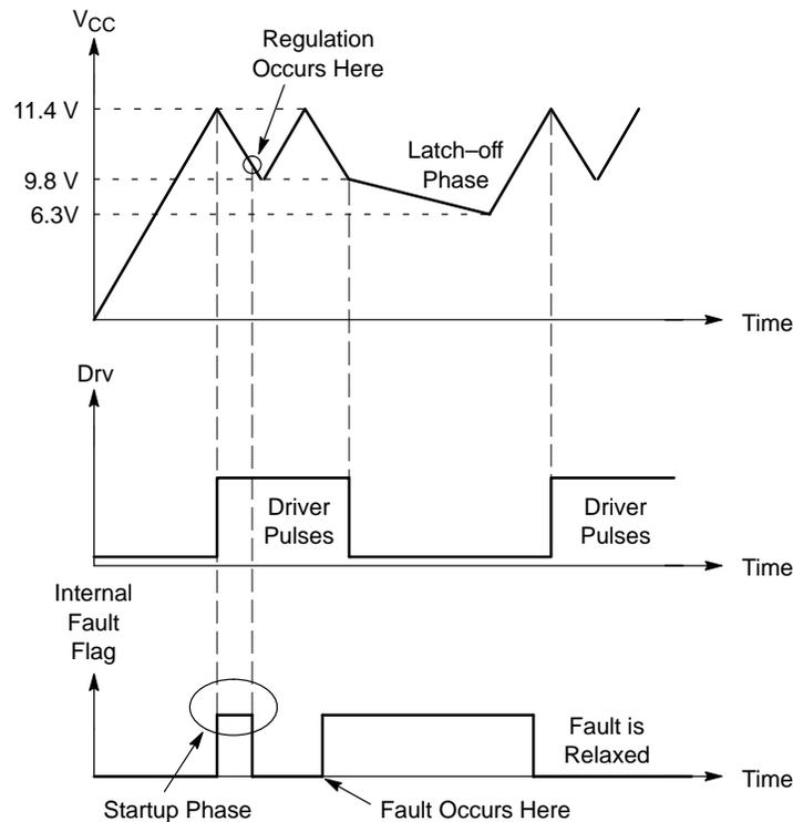
**Figure 5. If the fault is relaxed during the  $V_{CC}$  natural fall down sequence, the IC automatically resumes. If the fault still persists when  $V_{CC}$  reached  $UVLO_L$ , then the controller enters burst mode until recovery.**
