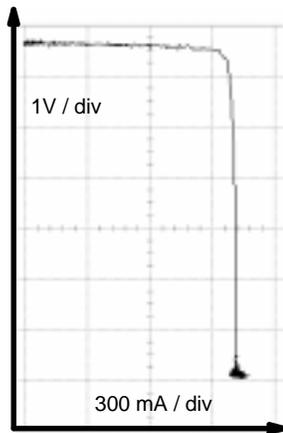
Figure 12f. The Resulting I-V Curve of the NCP1200 Charger Demoboard
