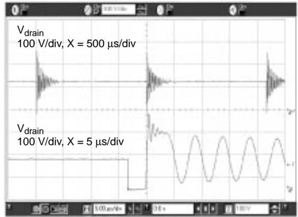
**Figure 11g. Standby operation, upper curve is V<sub>drain</sub> with X = 500 μs/div.**
