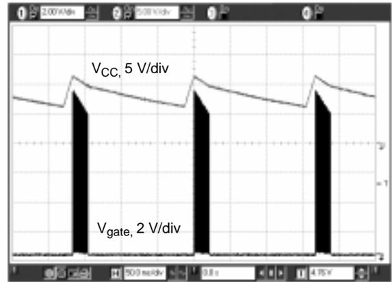
**Figure 11h. Typical Operating Curves in Short-Circuit Conditions**
