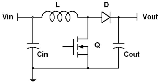
Figure 4. Conventional Boost Solution Schematic
