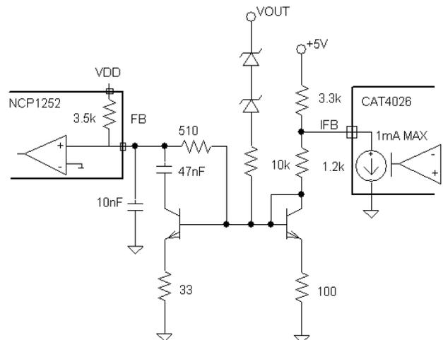
**Figure 31. Feedback Circuit**
