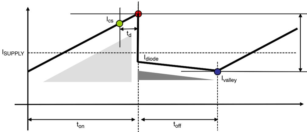
Figure 7. Tapped Coil Boost Current in the Coil
