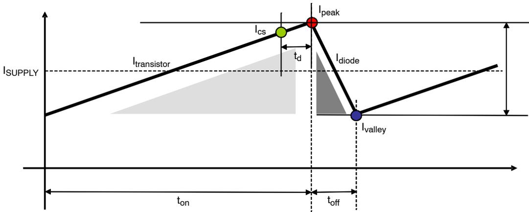
Figure 5. Conventional Boost Current in the Coil
