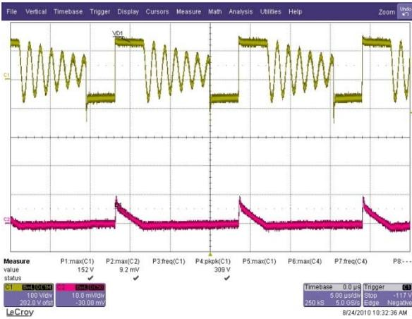
**Figure 15. Current in the Boost Diode D1**
