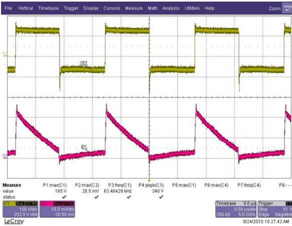
**Figure 12. Boost Diode D1 Current Waveform**
