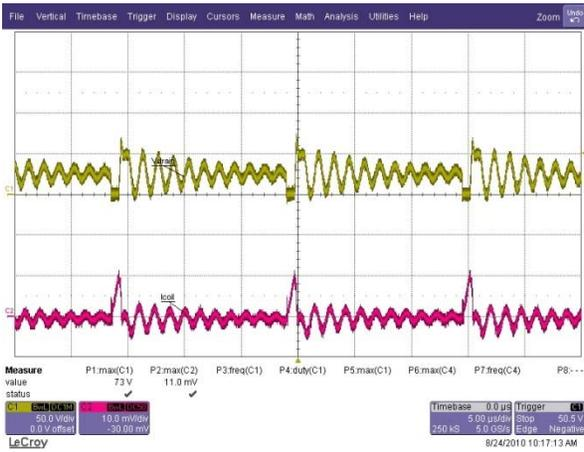
**Figure 18. Current in the Boost Coil**
