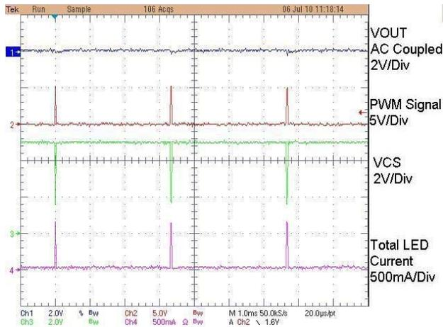
**Figure 20. PWM Waveforms 1% Duty Cycle**
