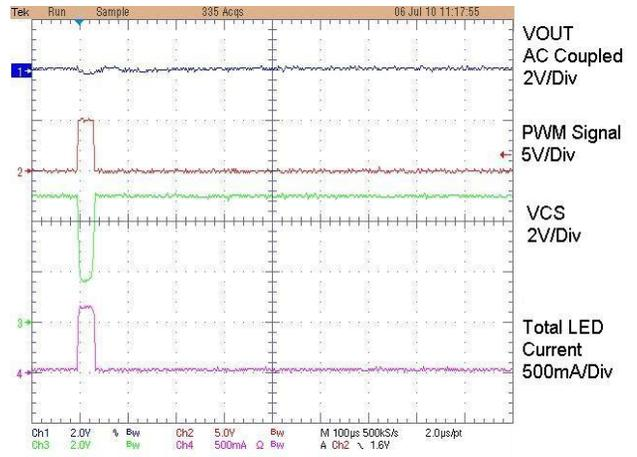
**Figure 21. PWM Waveforms 1% Duty Cycle Zoomed**
