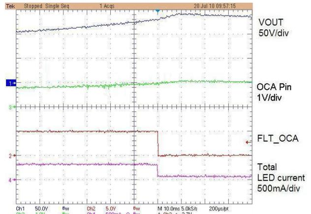
Figure 26. OCA Fault During Power Up
