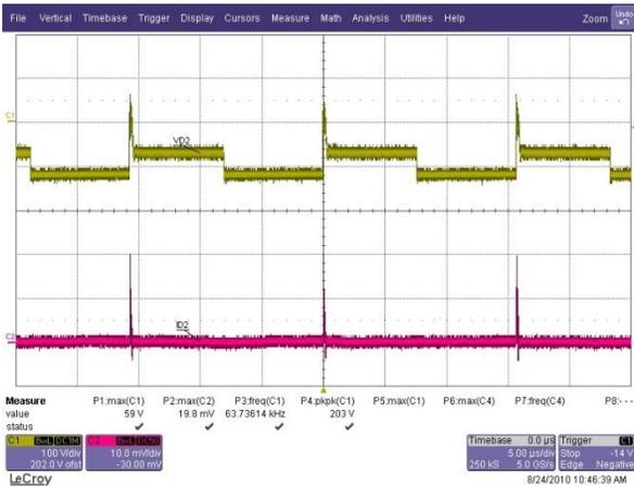
**Figure 16. Current in the Tapped Boost Diode D2**
