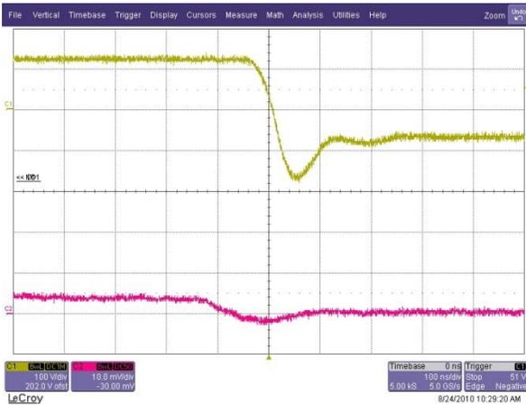
**Figure 13. Boost Diode D1 Switch OFF Waveform**
