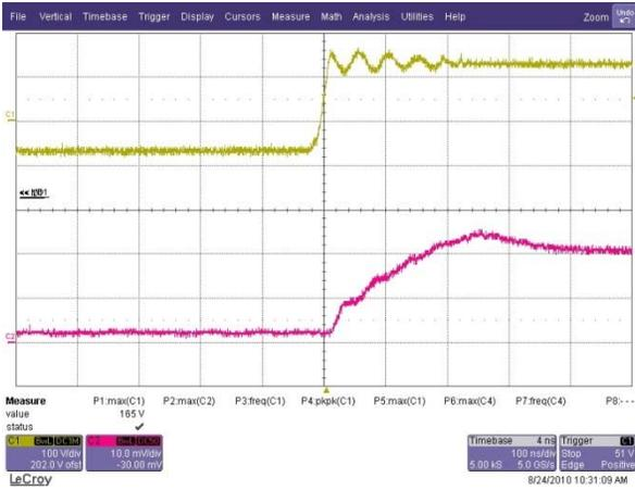
**Figure 14. Boost Diode D1 Switch ON
