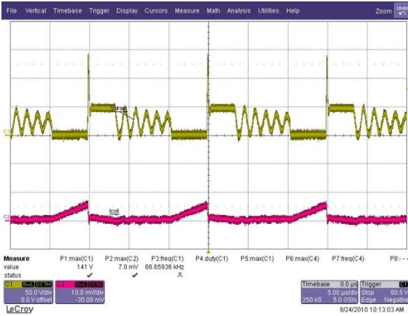
**Figure 11. Boost Coil Current Waveform**
