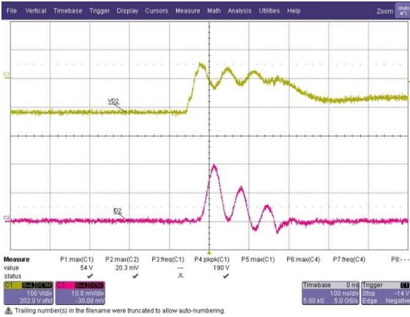
**Figure 17. Current in the Tapped Boost Diode D2**
