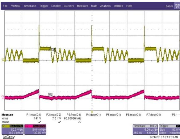
**Figure 10. Boost Coil Current Waveform**
