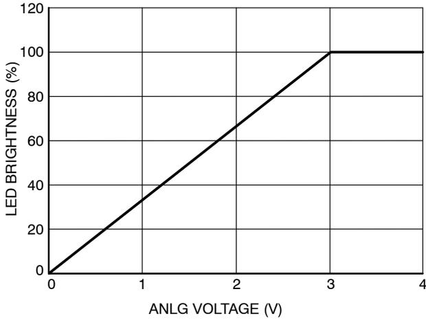
Figure 24. LED Brightness vs. ANLG Pin Voltage
