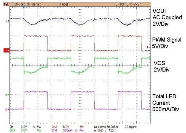
**Figure 22. PWM Waveforms 50% Duty Cycle**
