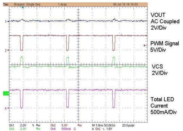
**Figure 23. PWM Waveforms 95% Duty Cycle**
