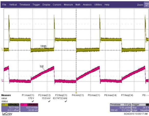
**Figure 9. Boost Coil Current Waveform**
