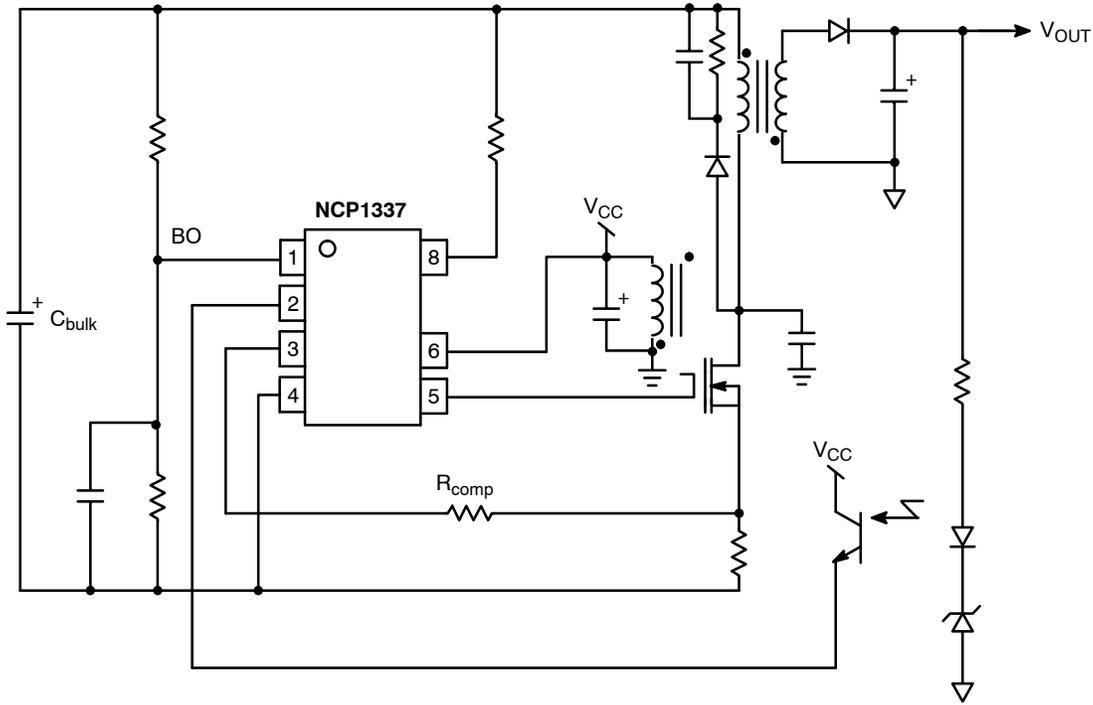
Figure 1. NCP1337 Typical Application Example
