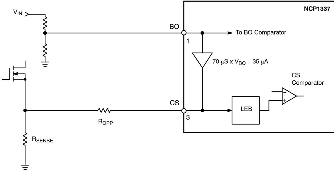
Figure 9. Internal Overpower Compensation Circuitry on CS Pin
