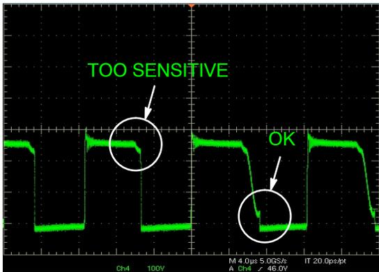
Figure 13. Instability with Multiple Outputs
