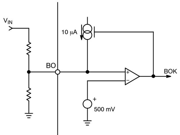
Figure 2. Internal Configuration of BO Protection
