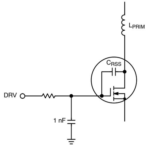
Figure 14. Gate-to-Ground Capacitor
