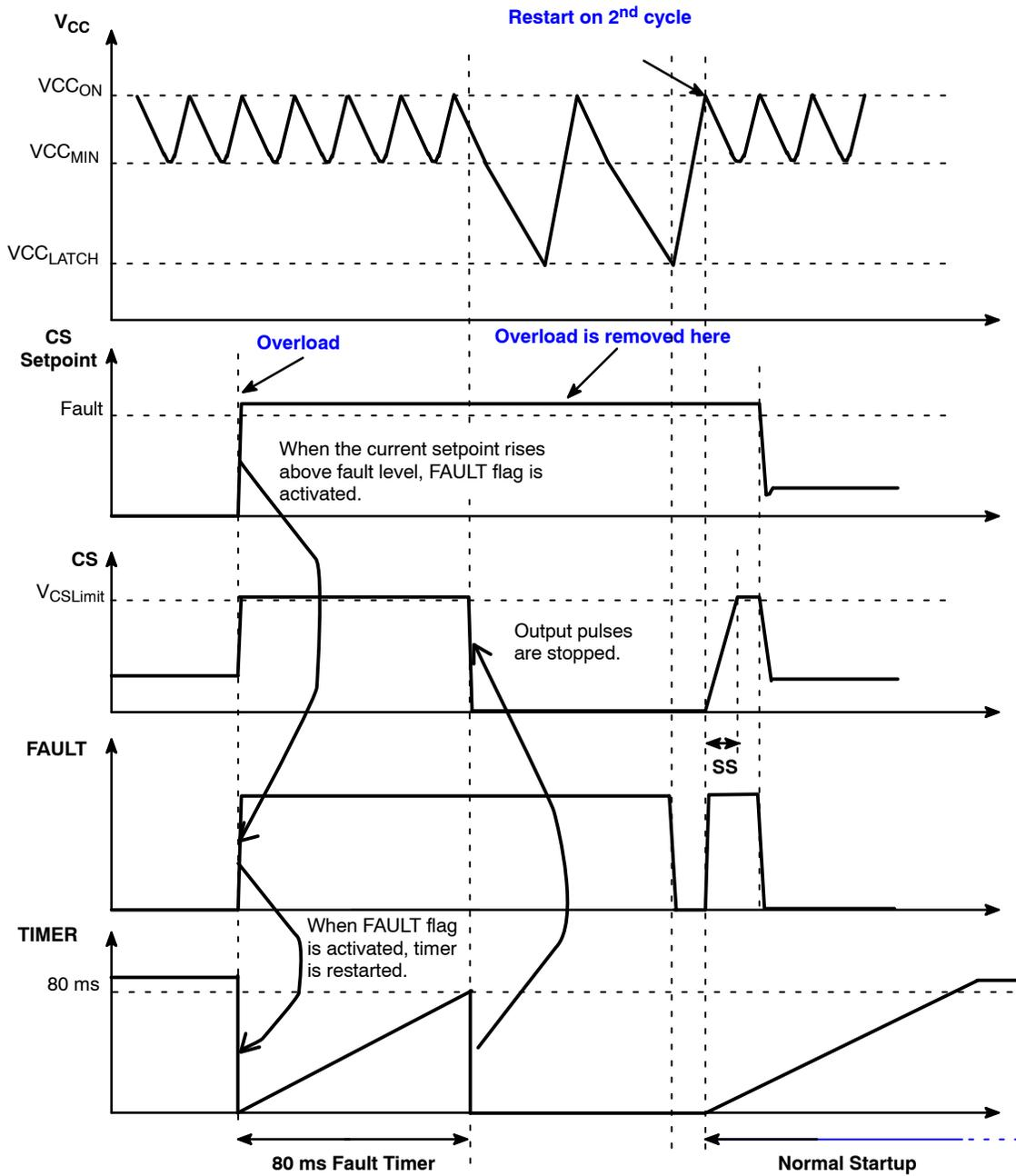
Figure 6. Typical Behavior in Overload Conditions
