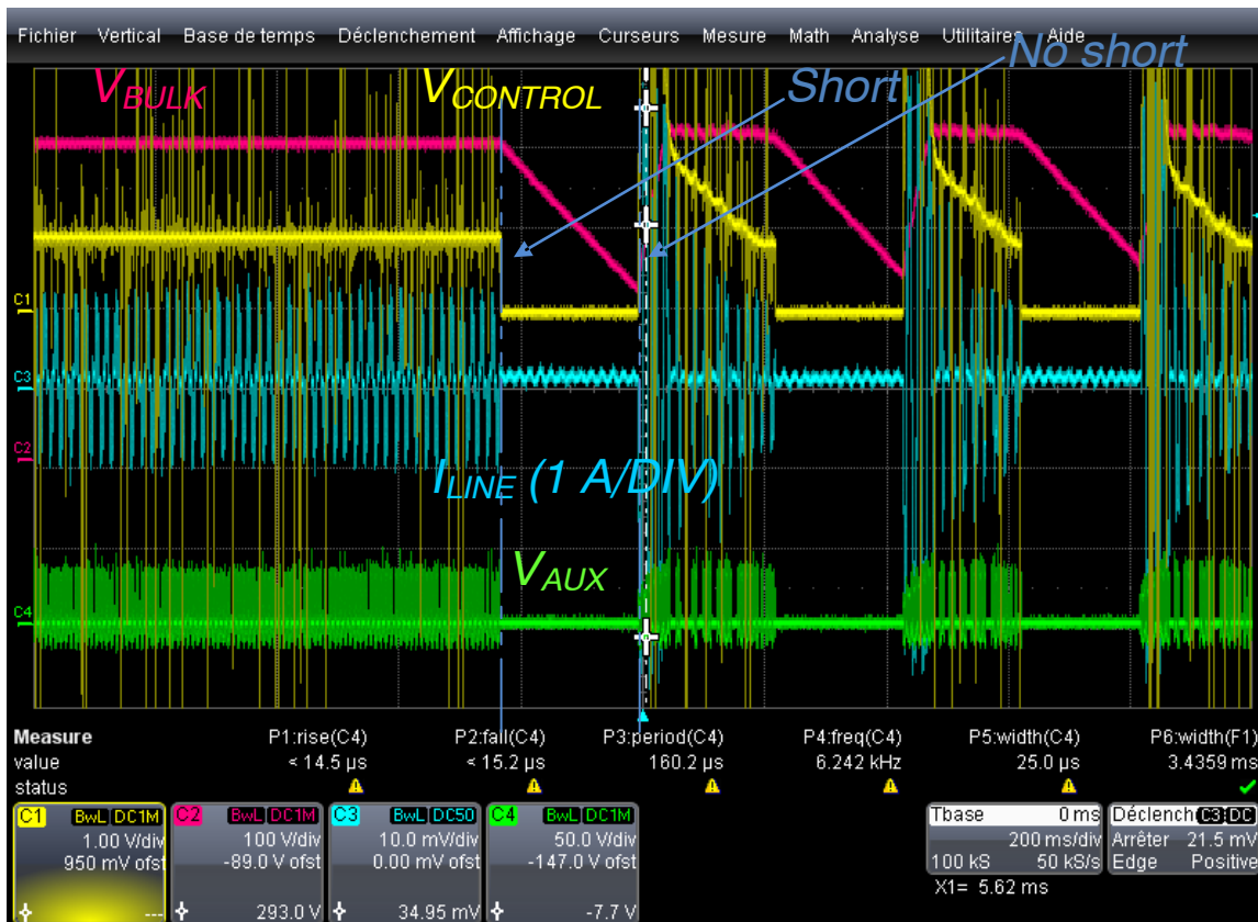
Figure 9. Intermittent Groundings/Releases of the V_{CONTROL} Pin
