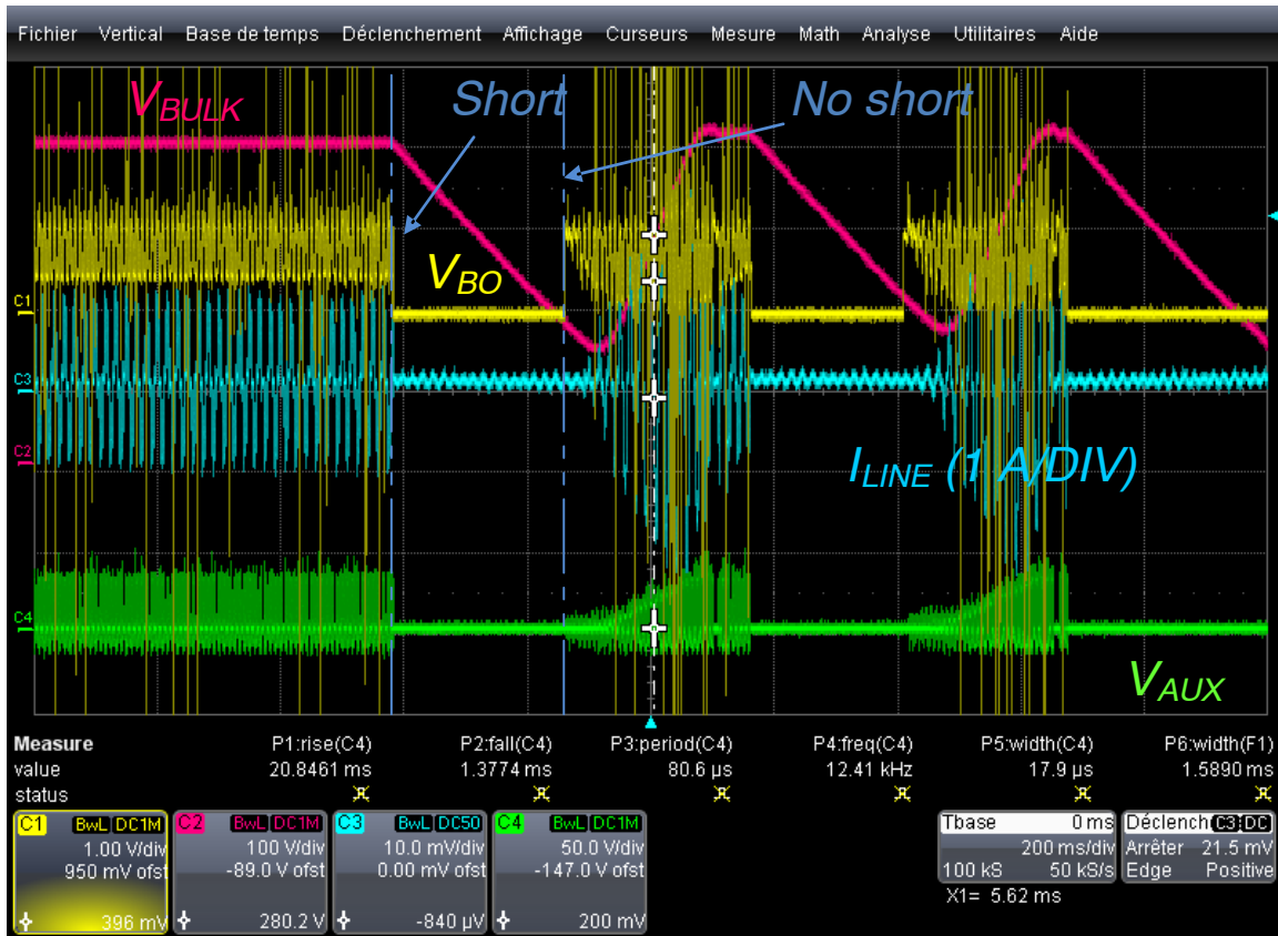
Figure 10. Intermittent Groundings/Releases of the V_{SENSE} Pin
