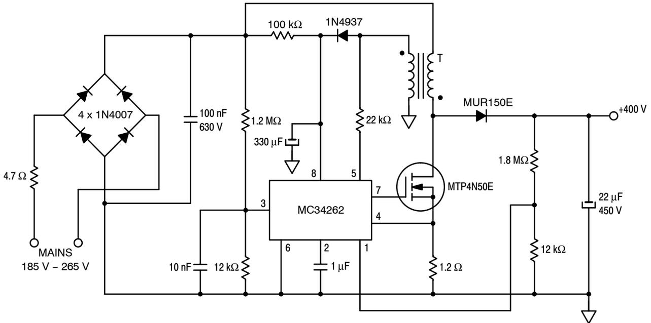
Figure 23. Typical PFC Circuit
