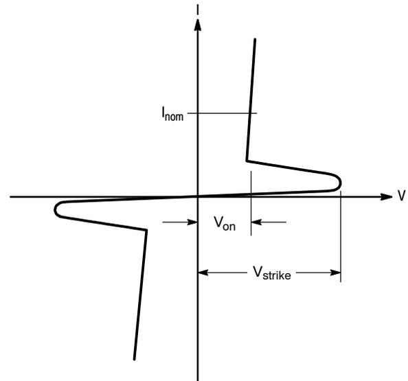
Figure 1. Typical Low Pressure Fluorescent Tube I/V Characteristic
