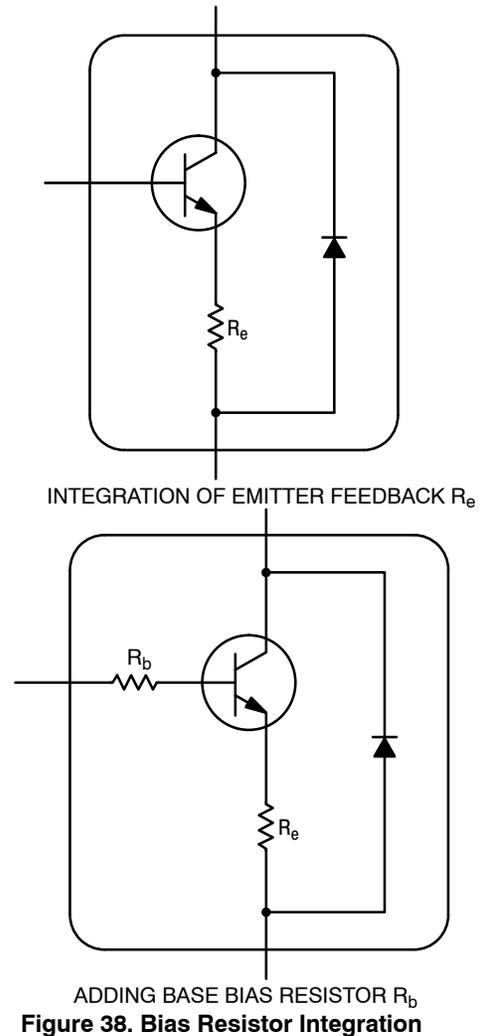
Figure 38. Bias Resistor Integration
