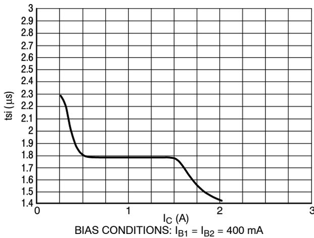
Figure 35.  $t_{si} = f(I_C)$  at  $I_{B1} = I_{B2} = \text{Constant}$
