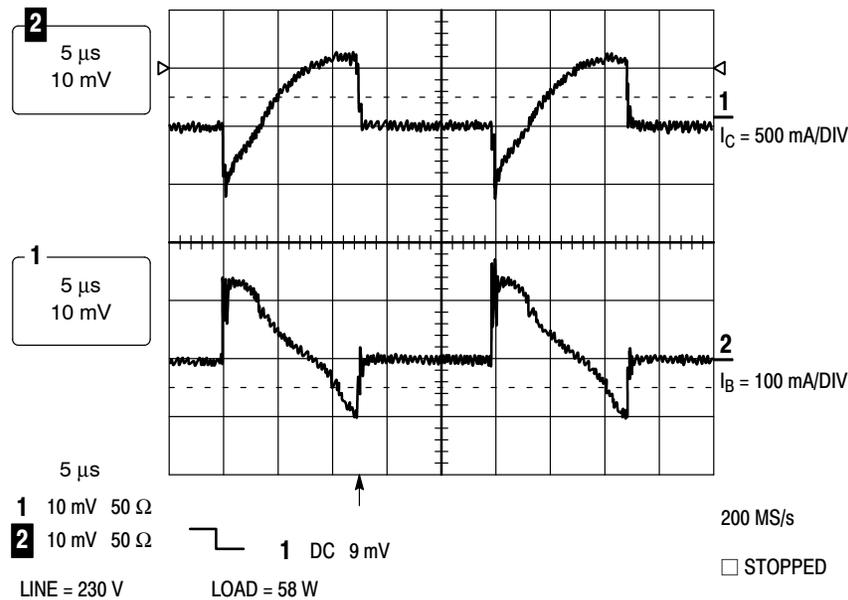
**Figure 26. Collector and Base Currents in Steady State**
