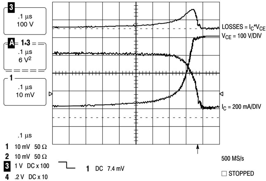
Figure 27. Switching Losses
