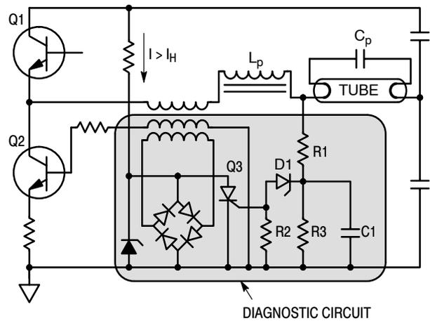
Figure 21. Fault Memorization
