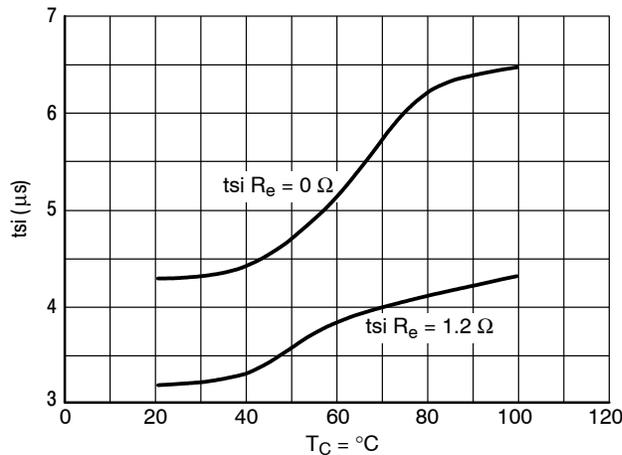
Figure 36.  $t_{si} = f(T_C)$  at  $I_C = \text{Constant}$
