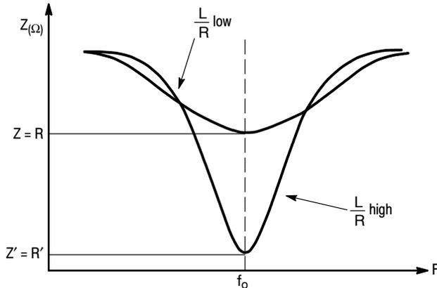
Figure 12. Typical R/L/C Series Network Behavior
