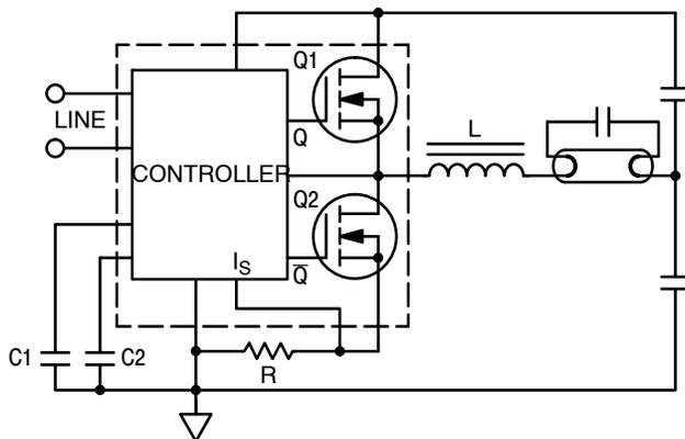
**Figure 45. Fully Integrated Low Power Electronic Lamp Ballast**
