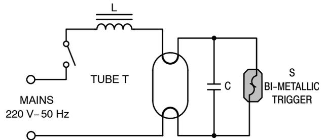
**Figure 3. Standard Ballast Circuit for Fluorescent Tube**
