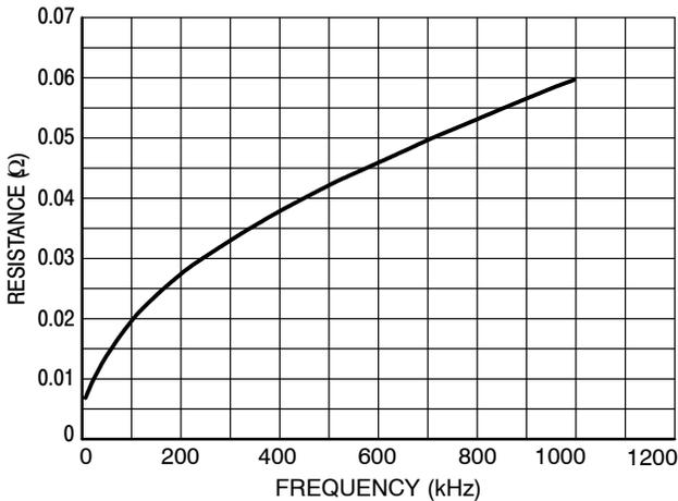
NOTE: Wire is solid copper, one meter long, diameter 2.00 mm, temperature is +20°C.
