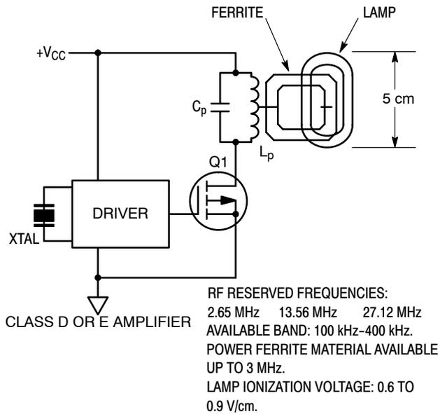
**Figure 47. Typical Static Induction Discharge Lamp Application**
