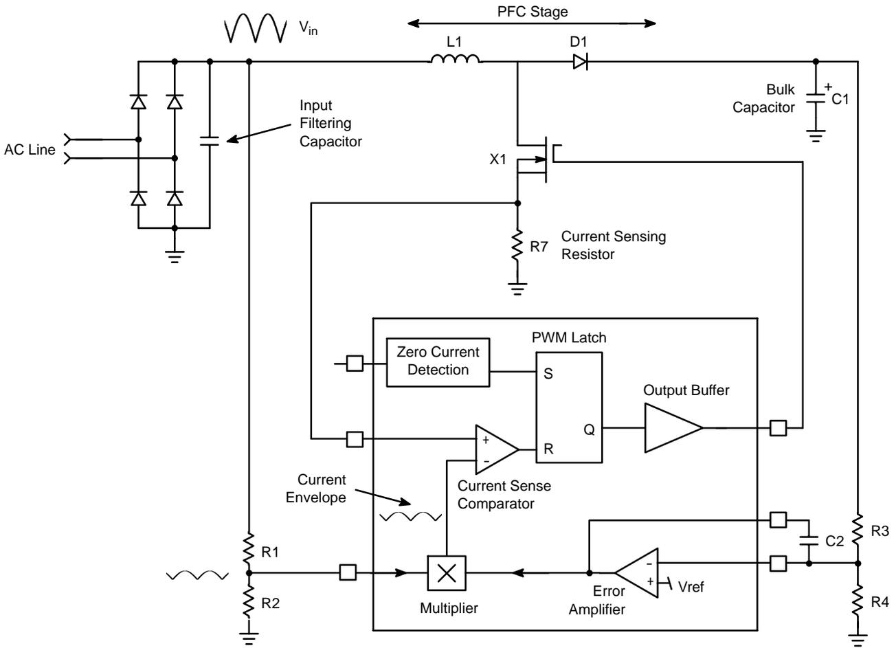
**Figure 3. Switching Sequences of the PFC Stage**
