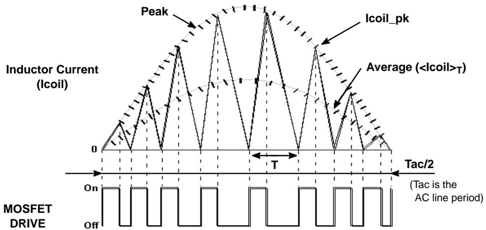
**Figure 4. Coil Current**
