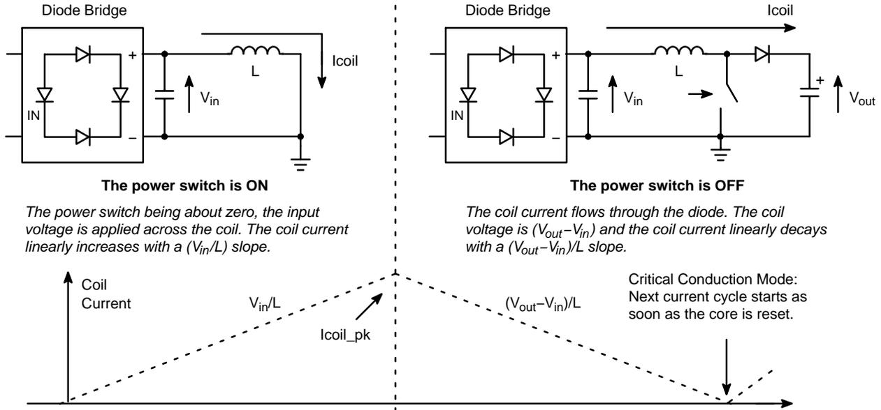
Figure 2. Switching Sequences of the PFC Stage
