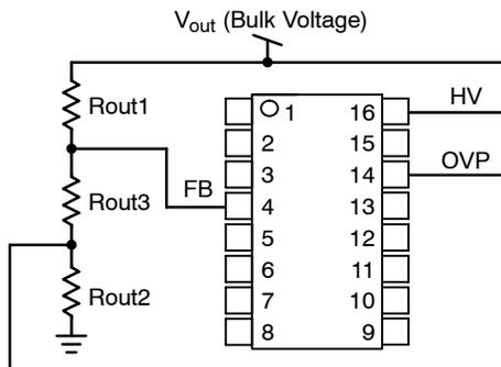
Figure 7. Configuration with One Feed-back Network for Both OVP and Regulation
