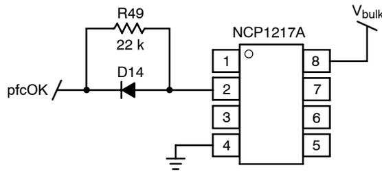
Figure 12. Enabling / Disabling the Downstream Converter
