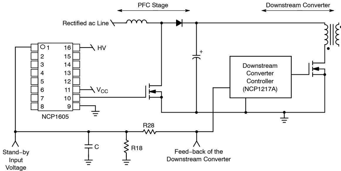
Figure 10. Signal for Stand-by Detection
