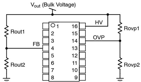
Figure 8. Configuration with Two Separate Feed-back Networks
