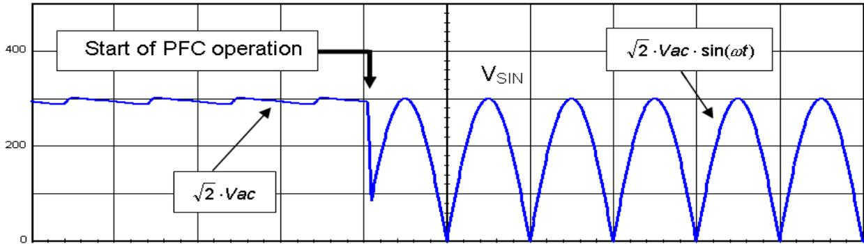
Figure 4. Typical Input Voltage of a PFC Stage
