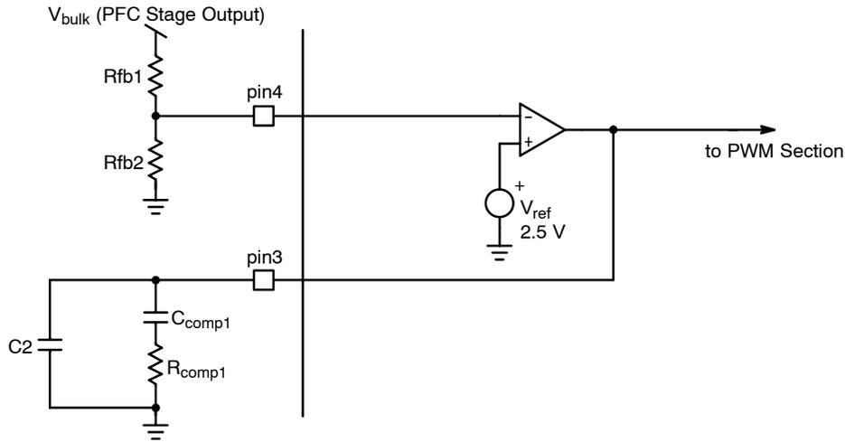
Figure 5. Regulation Trans-conductance Error Amplifier, Feed-back and Compensation Network
