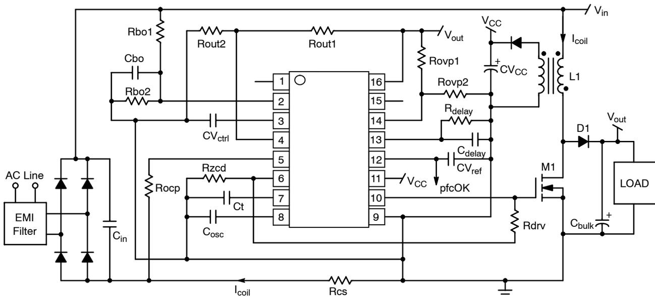
Figure 1. Generic Application Schematic
