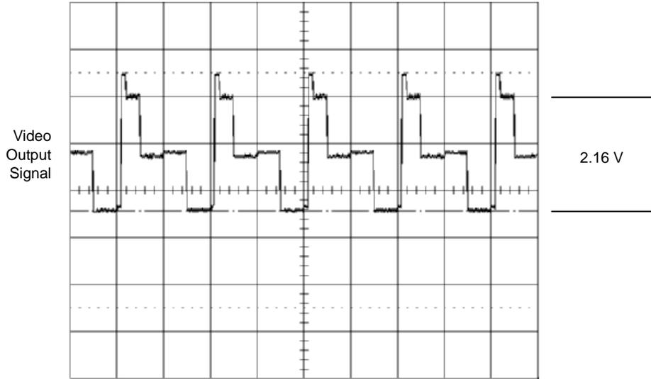
**Figure 14. Floating Diffusion Charge Capacity (Nominal Settings)**
