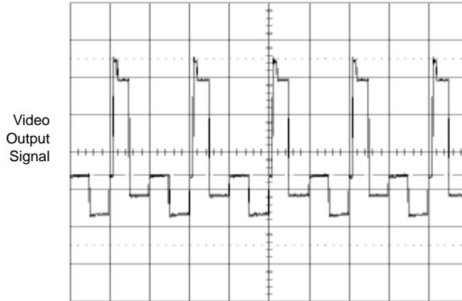
**Figure 16. Output Video when Charge Flows Back Over the Output Gate**
