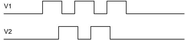
Figure 3. Vertical Timing to Combine Two Lines
