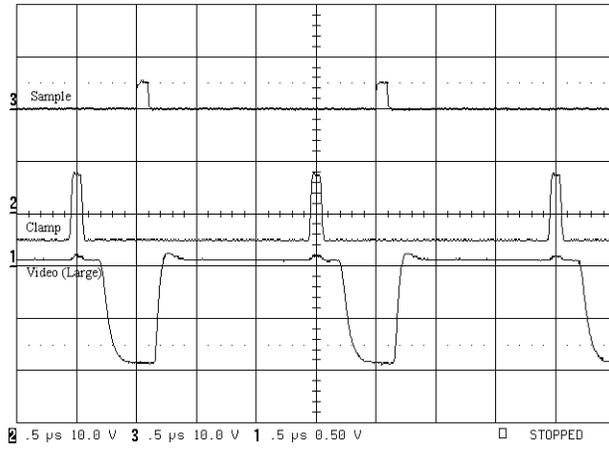
Figure 8. Two Columns Binned on to H21 (Sample/Clamp/Vid)
