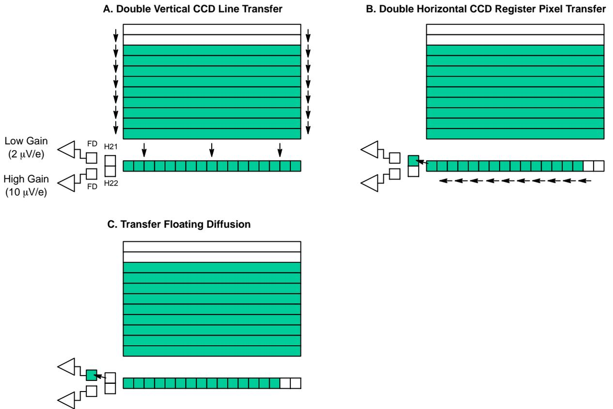
Figure 12. Charge Transport: 2x2 Binning on Transfer Gate (H21) Using Low Gain (2  $\mu\text{V}/\text{electron}$ ) Output
