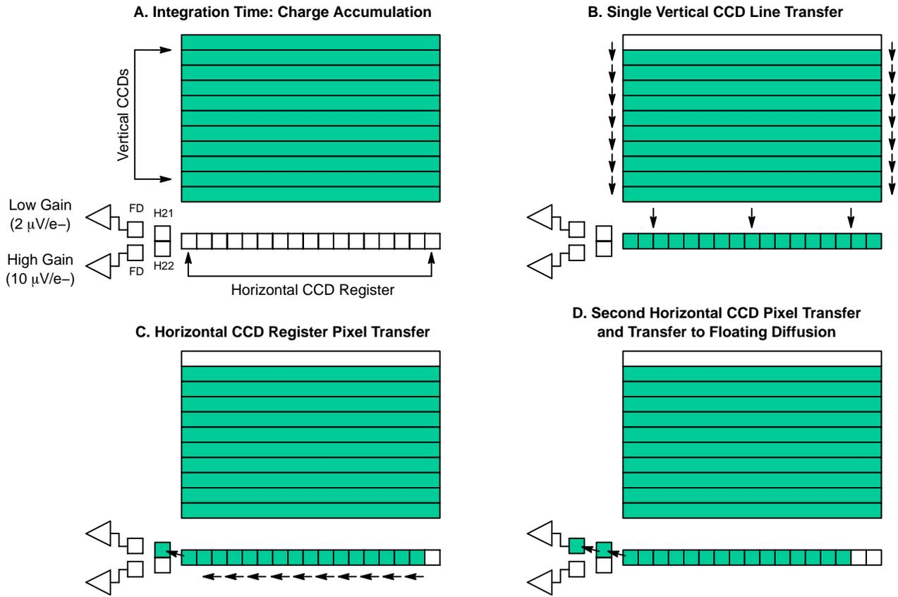
Figure 1. Normal Readout through Low Gain Output
