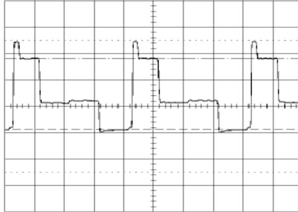
Figure 18. Charge Lost Over the Reset Gate
