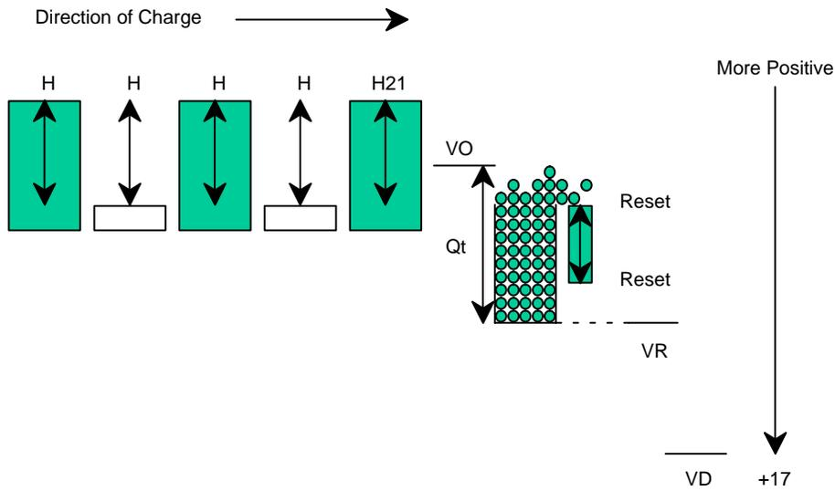
Figure 19. Charge Lost Over the Reset Gate
