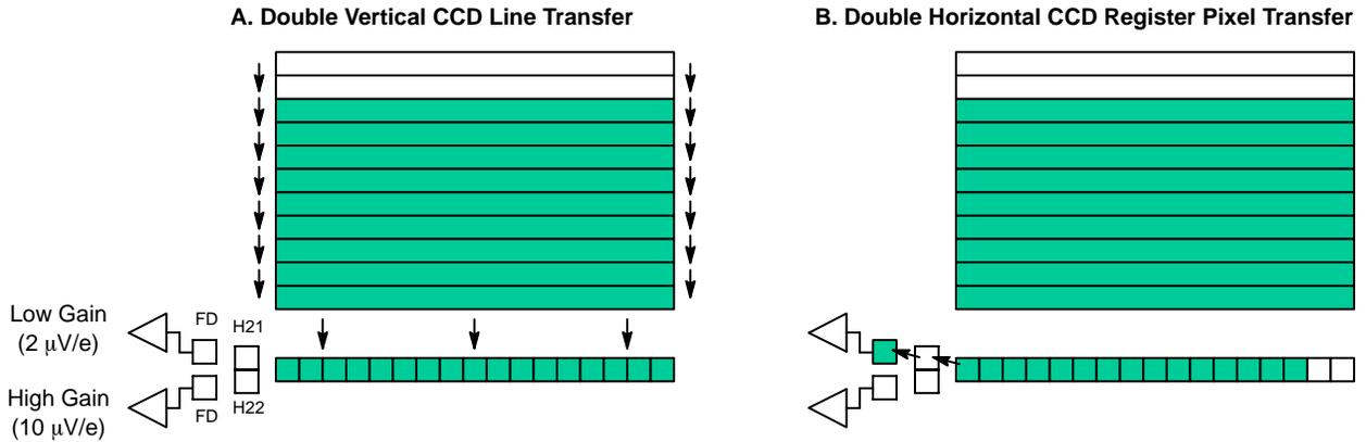
Figure 11. Charge Transport: 2x2 Binning on Floating Diffusion Using Low Gain (2  $\mu\text{V}/\text{electron}$ ) Output
