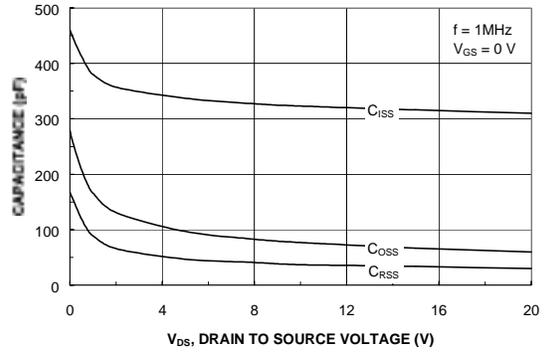
**Figure 8. Capacitance Characteristics.**
