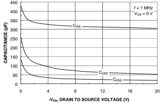
**Figure 18. Capacitance Characteristics.**
