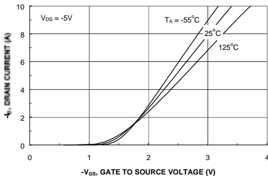
Figure 15. Transfer Characteristics.
