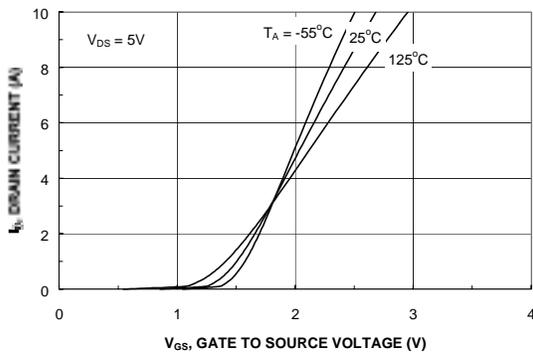
Figure 5. Transfer Characteristics.
