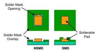
Figure 3. Comparison of NSMD vs. SMD Pads
