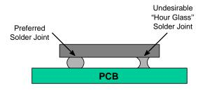
Figure 8. Side View of QFN Attachment Illustrating Preferred and Undesirable Solder Joint Shapes
