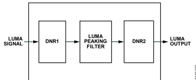
Figure 23. DNR and Peaking Block Diagram
