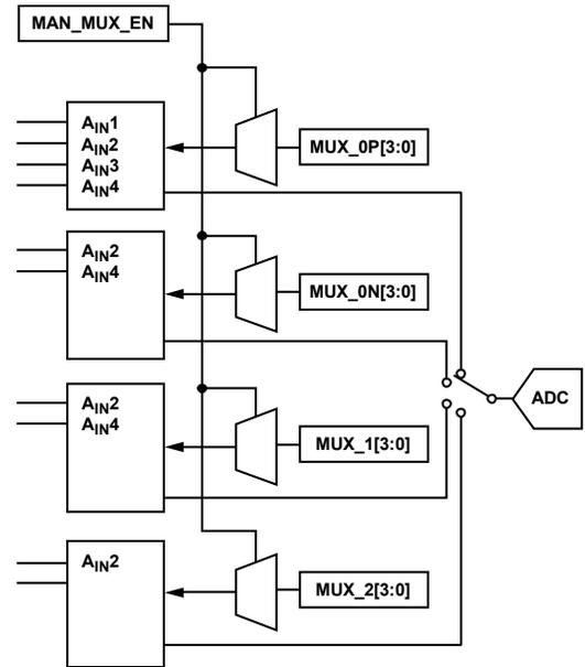
Figure 3. Manual Muxing Scheme for [ADV7282A](#)
