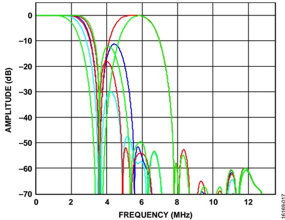
Figure 17. Combined Y Antialias Filter, NTSC Notch Filter, and Y Resample
