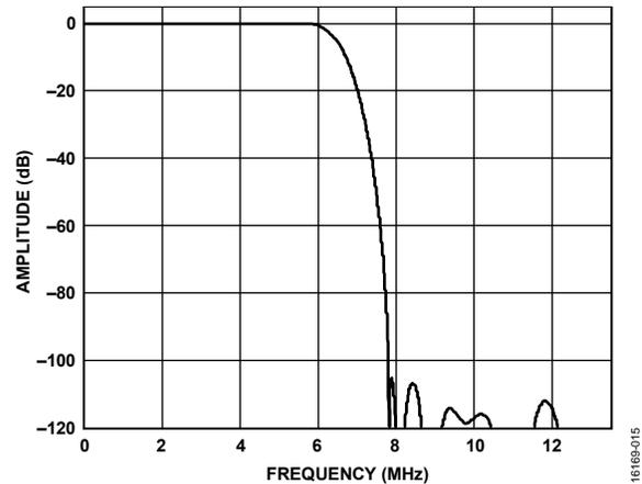
Figure 15. Combined Y Antialias, CCIR Mode Shaping Filter, Y Resample Responses
