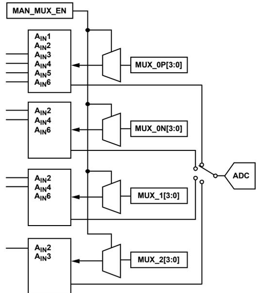
Figure 4. Manual Muxing Scheme for [ADV7281A-M](#) and [ADV7282A-M](#)
