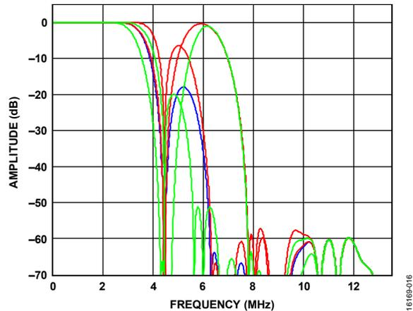
Figure 16. Combined Y Antialias, PAL Notch Filters, and Y Resample Responses
