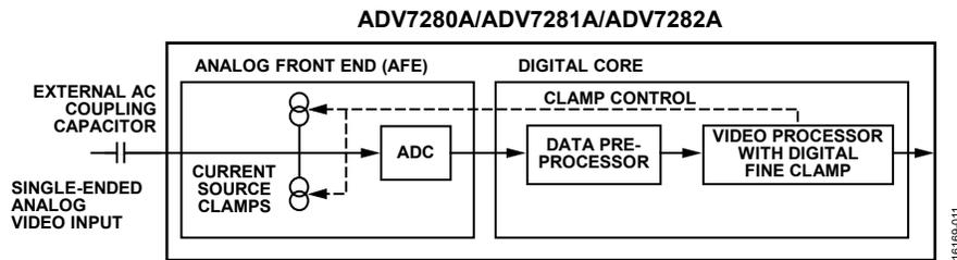
Figure 11. Single-Ended Clamping Overview
