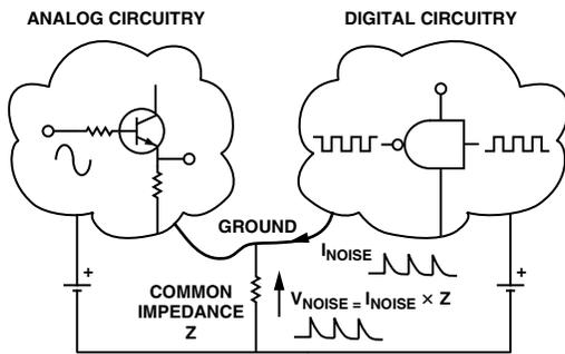
Figure 25. Noise Coupling via Ground Return Impedance
