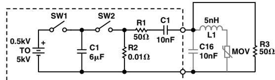
Figure 17. EFT Generator
