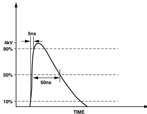
Figure 15. Single EFT Pulse Characteristics
