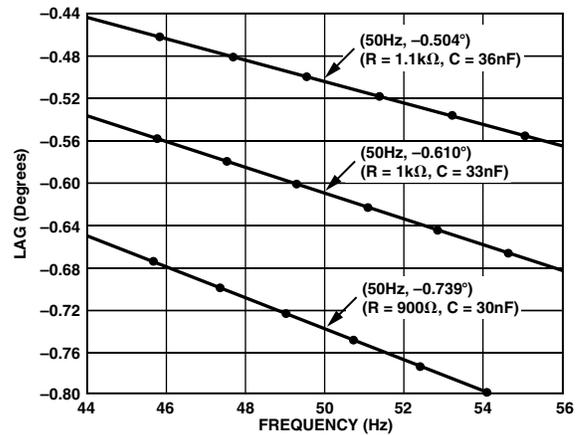
Figure 9. Phase Shift at 50 Hz Due to Component Tolerances
