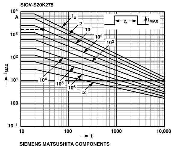
Figure 24. Derating Curve for S20K275
