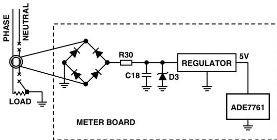
Figure 12. Current Transformer Supply (PS2)
