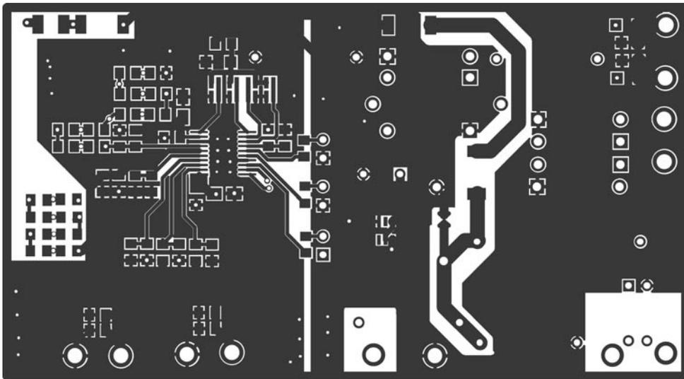
Figure 30. PCB (Bottom Layer)
