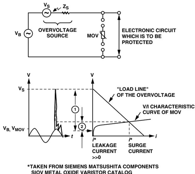
Figure 16. Principle of MOV Overvoltage Protection
