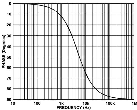
Figure 8. RC Phase Filter Response
