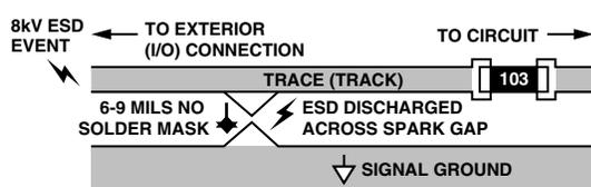
Figure 13. Spark Gap to Arrest ESD Events
