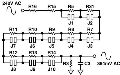
Figure 4. Line Attenuation Network
