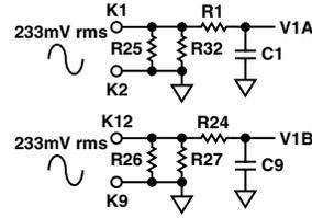
Figure 2. Current Input Network
