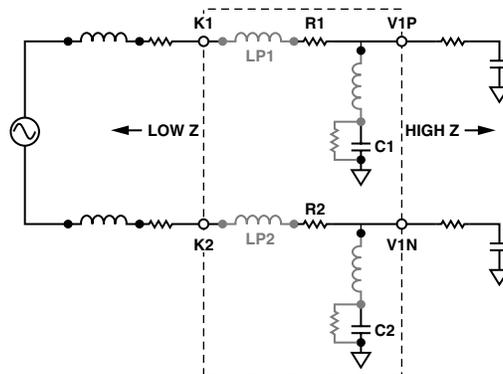
Figure 14. Anti-Alias Filters Showing Parasitics
