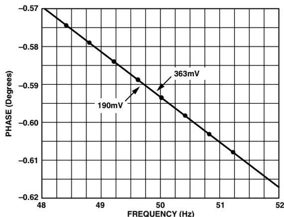
Figure 10. Phase Shift Due to Calibration
