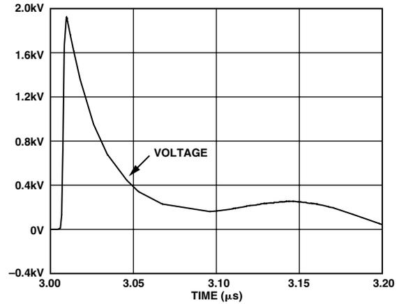
Figure 20. EFT Generator Output into 50 Ω with MOV in Place and Stray Inductance of 1 μH
