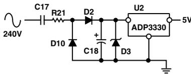
Figure 11. Capacitor Divider Supply (PS1)
