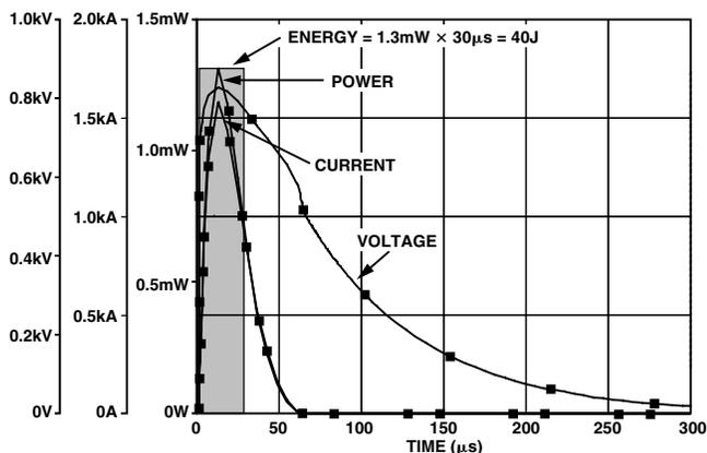
Figure 23. Energy Absorbed by MOV During 4 kV Surge
