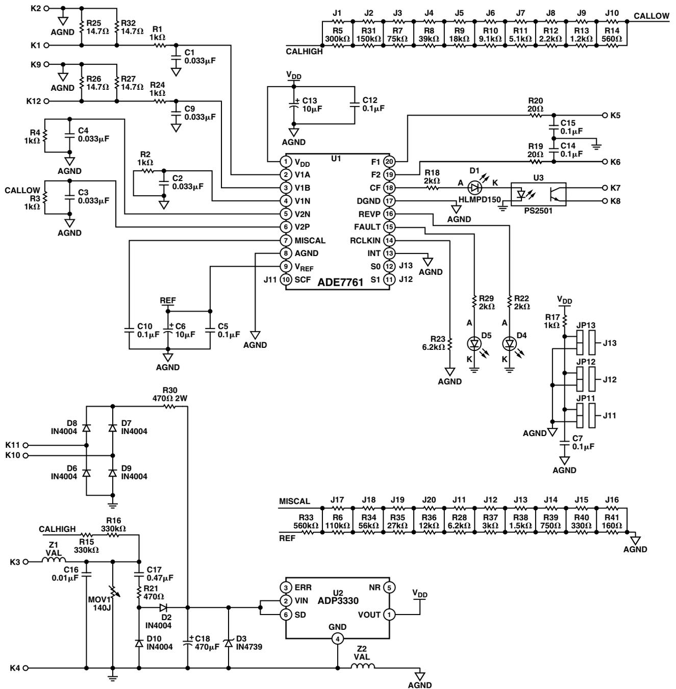
Figure 31. ADE7761 Reference Design Schematic
