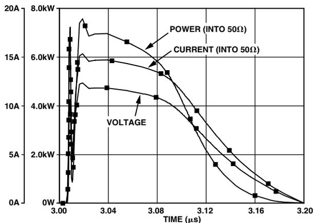
Figure 19. EFT Generator Output into 50 Ω with MOV in Place
