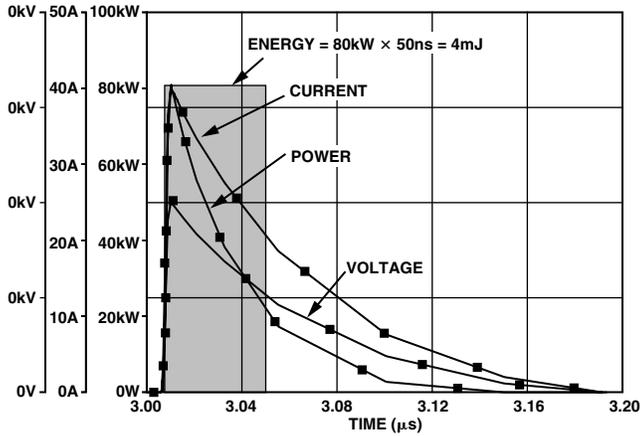
Figure 18. EFT Generator Output into 50 Ω (No Protection)
