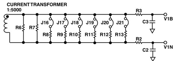
Figure 3. Calibration Network for V1A and V1B Mismatch
