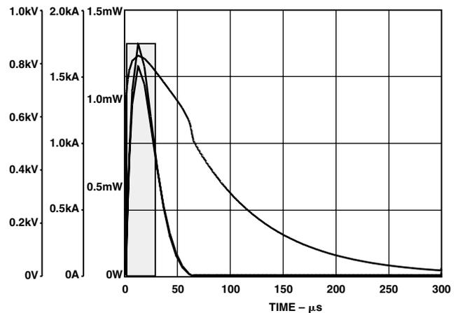
Figure 32. Energy Absorbed by MOV During 4 kV Surge
