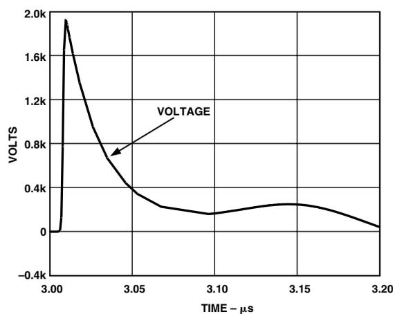
Figure 28. EFT Generator Output into 50 Ω with MOV in Place and Stray Inductance of 1 µH
