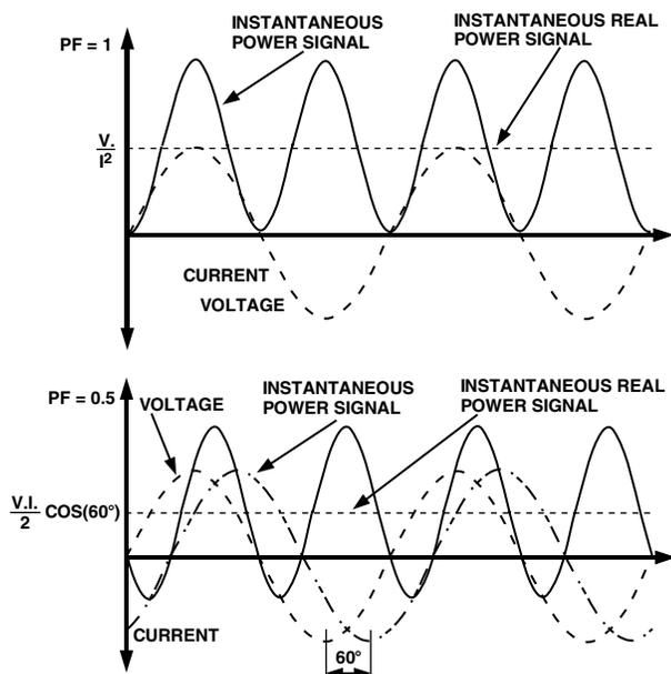
Figure 4. Voltage and Current Waveform (Inductive Load)
