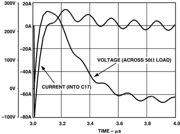
Figure 29. EFT Generator Output into 50 Ω with MOV and C17 (10 nF) in Place and Stray Inductance of 1 μH
