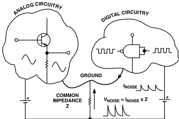
Figure 34. Noise Coupling via Ground Return Impedance
