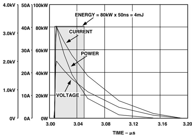
Figure 26. EFT Generator Output into 50 Ω (No Protection)
