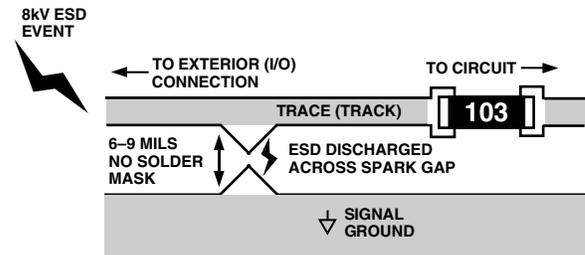
Figure 19. Spark Gap to Arrest ESD Events
