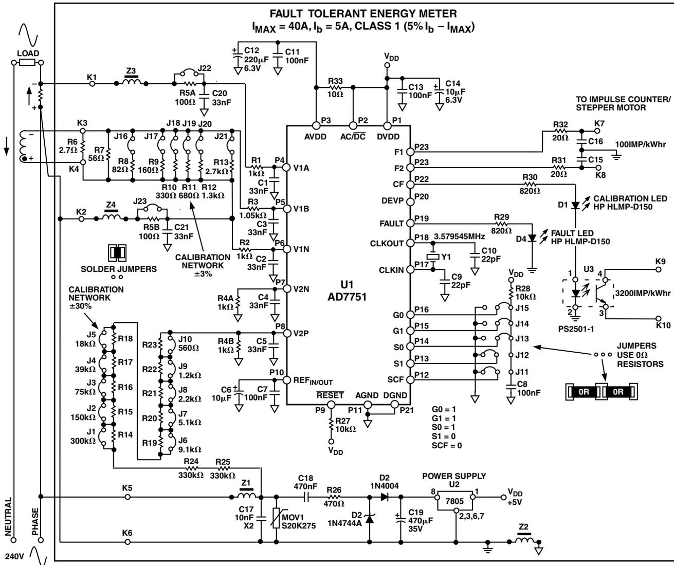
Figure 1. Tamper-Resistant Single Phase Watt-Hour Meter Based on the AD7751
