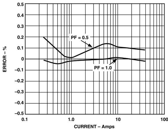
Figure 36. Measurement Error (% Reading, 240 V, 50 Hz)
