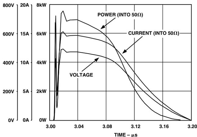
Figure 27. EFT Generator Output into 50 Ω with MOV in Place
