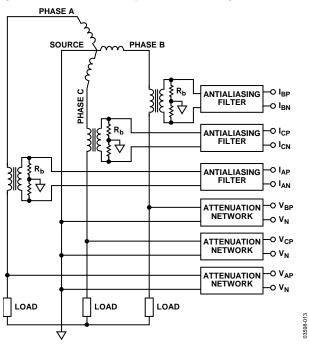
Figure 13. 4-Wire Wye with Three Voltage Sensors
