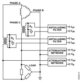
Figure 15. 3-Wire Delta Configuration
