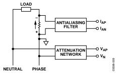
Figure 9. Single-Phase, One Current Sensor
