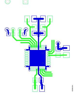
Figure 4. ADE7878 Top Layer Printed Circuit Board
