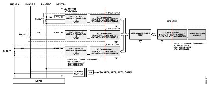
Figure 17. Single-Phase ADE ICs in a Three-Phase Application
