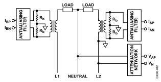
Figure 12. Split-Phase, Two Current Sensors
