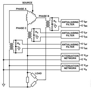
Figure 16. 4-Wire Delta Configuration
