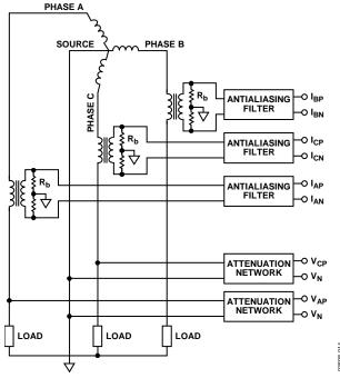
Figure 14. 4-Wire Wye with Two Voltage Sensors
