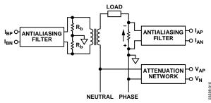
Figure 10. Single-Phase, Two Current Sensors
