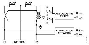
Figure 11. Split-Phase, One Current Sensor
