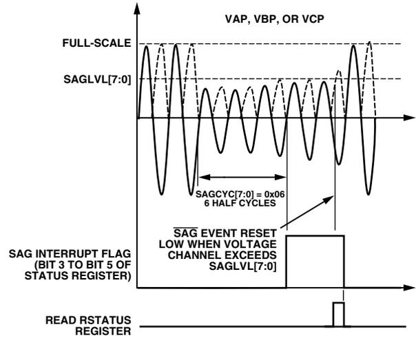
Figure 4. Voltage SAG Detection
