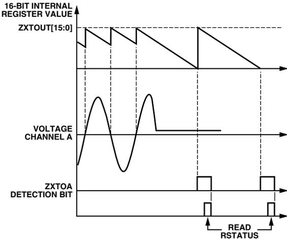
Figure 3. Zero-Crossing Timeout Detection
