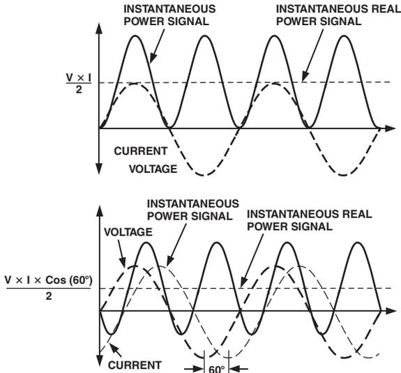
Figure 5. Voltage and Current (Inductive Load)
