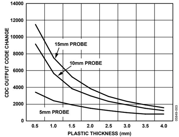
Figure 3. Button Sensor Response
