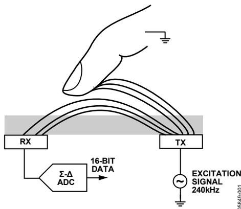
Figure 1. Capacitance Sensing
