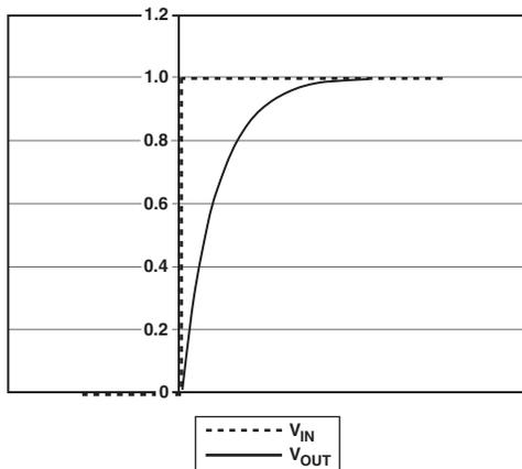
Figure 2. Analog Filter Step Response
