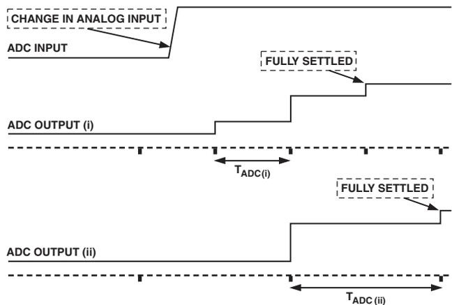
Figure 3. Comparison of ADC Latency with (i) and without (ii) Extra ‘Intermediate’ Results
