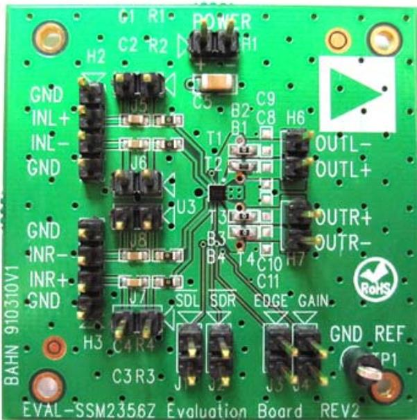
Figure 1. SSM2356 Evaluation Board Top View
