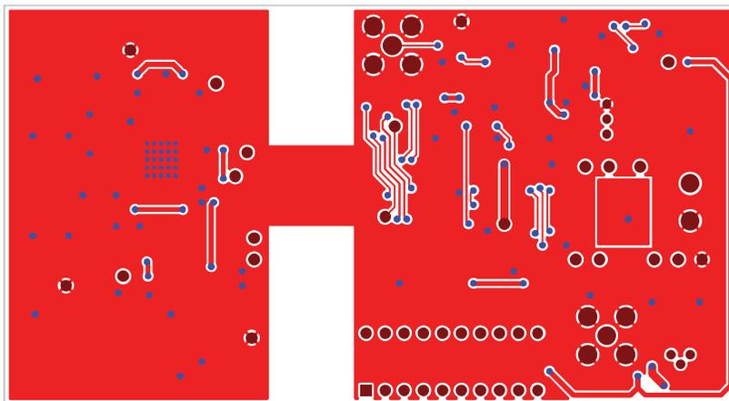
Figure 21. EVAL-ADT7516EBZ Evaluation Board PCB Layout (Solder Side)
