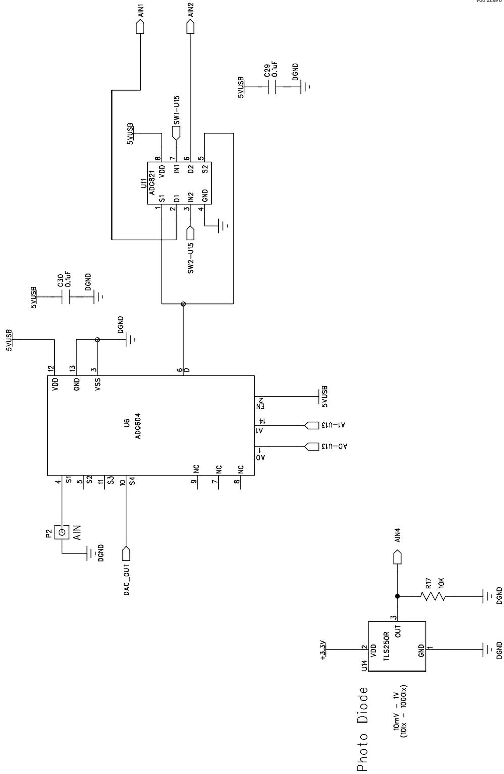
Figure 18. EVAL-ADT7516EBZ Evaluation Board Schematic Part 4
