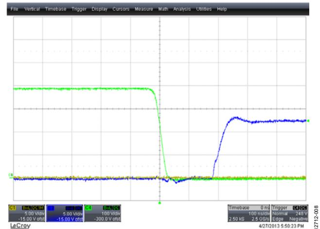
Figure 9. ZVS Transition at Heavy Load (Passive to Active)
