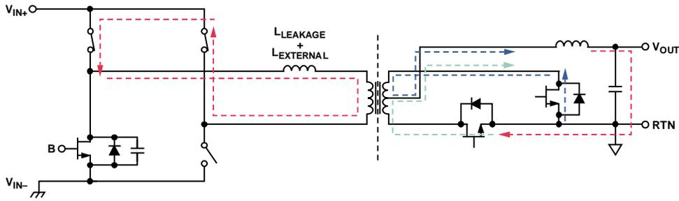
Figure 2. Active to Passive Stage That Shows ZVS of QC
