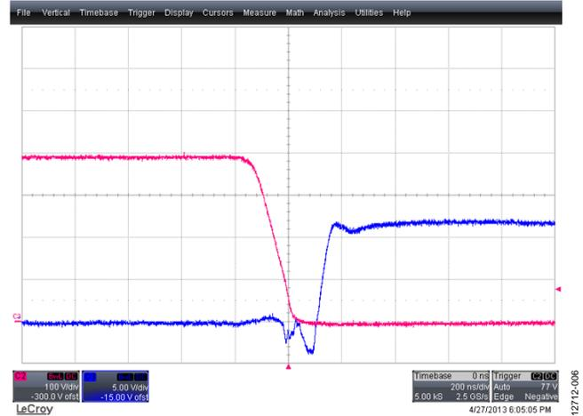
Figure 6. Slew Rate of the Falling Drain Voltage Across Switch  $Q_C$  at Half Load (Active to Passive Transition)
