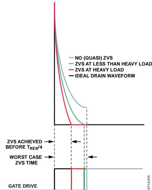
Figure 8. ZVS Transition at Various Loads
