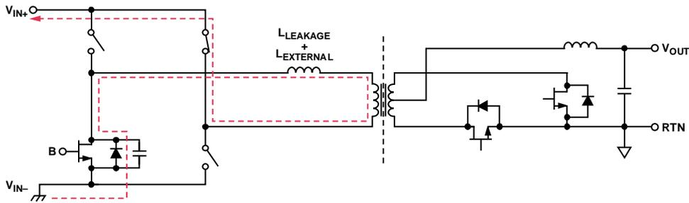
Figure 3. Passive to Active Stage That Shows ZVS of QB
