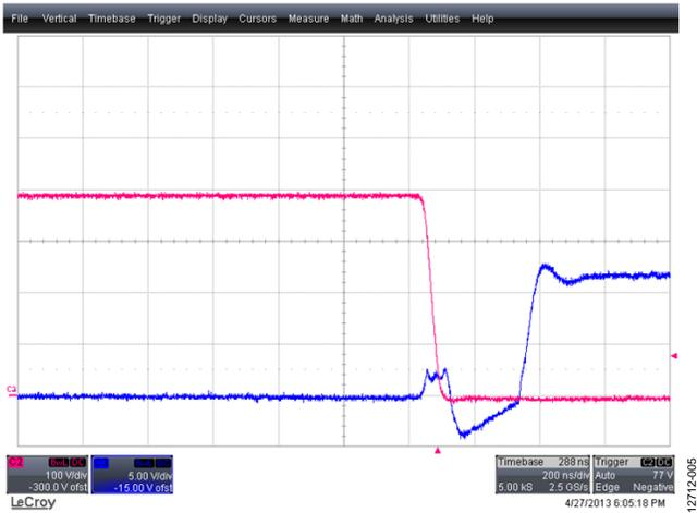
Figure 5. Slew Rate of the Falling Drain Voltage Across Switch  $Q_C$  at Heavy Load (Active to Passive Transition)
