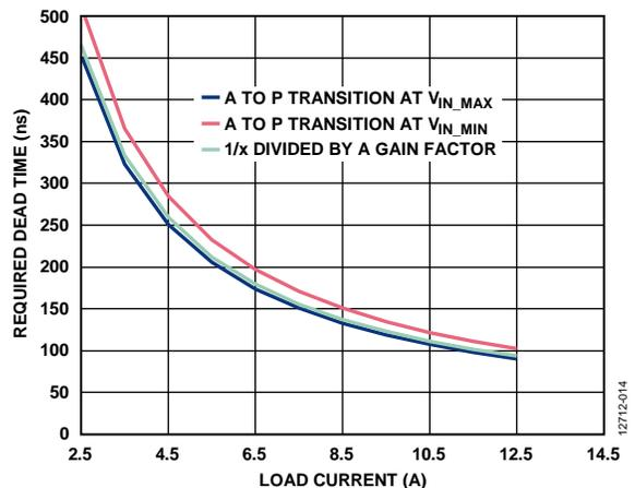
Figure 14. ZVS Transition Time During Active to Passive (A to P) Transition Based on Load Current
