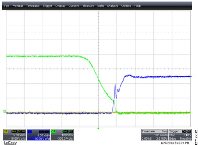
Figure 11. ZVS Transition at Light Load (Passive to Active)
