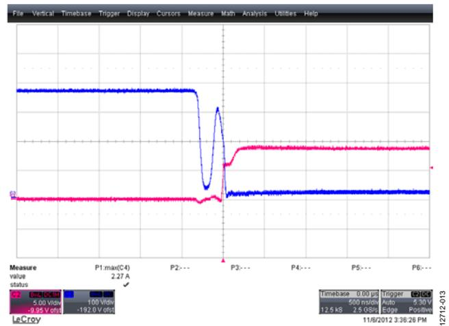
Figure 13. Nonoptimized ZVS Transition Time (Note That the Blue Trace Is the Switch Drain Voltage and the Red Trace Is the Gate Drive.)
