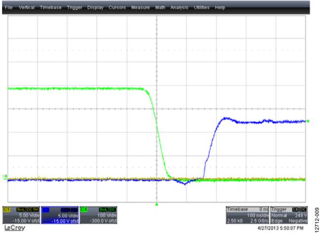
Figure 10. ZVS Transition at Half Load (Passive to Active)
