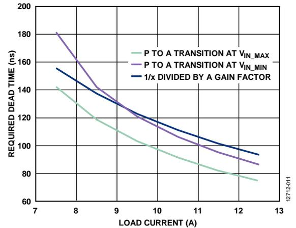
Figure 12. ZVS Transition Time During Passive to Active (P to A) Transition Based on Load Current
