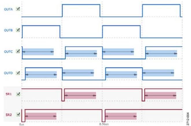
Figure 4. Typical PWM Setup for Full Bridge Phase Shifted Topology
