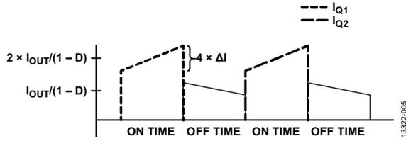
Figure 4. Idealized SEPIC Waveforms
