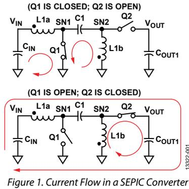
Figure 1. Current Flow in a SEPIC Converter
