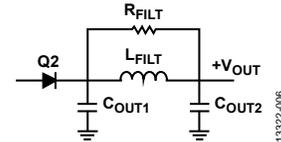
Figure 5. Schematic of the Output Filter
