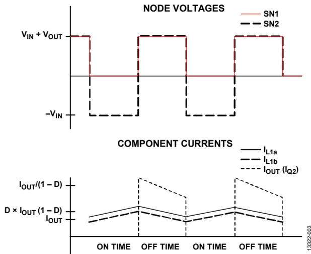
Figure 2. Idealized SEPIC Waveforms
