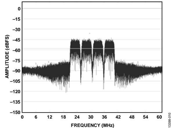
Figure 10. Intermodulation Products Obscured by Noise Shaping
