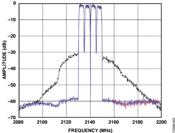
Figure 2. Uncorrected Amplifier ACPR
