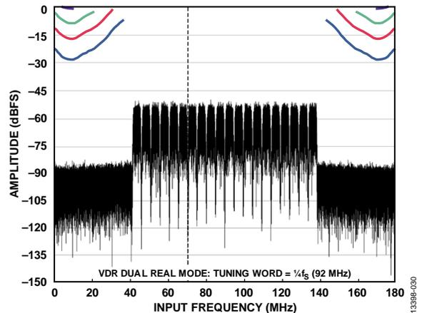
Figure 30. VDR Real Mode ( $1/4 f_s$  Tuning) with Multicarrier LTE Signal Overlay
