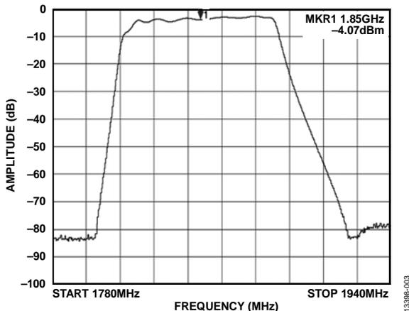
Figure 3. Typical Transmit Filter Response
