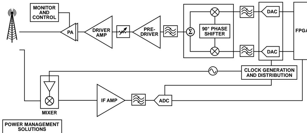
Figure 1. Typical DPD System Diagram
