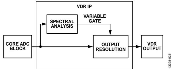
Figure 25. VDR Signal Flow Diagram
