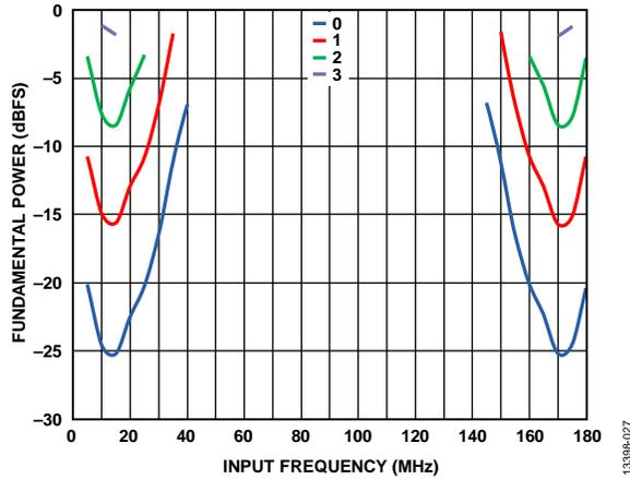
Figure 27. Frequency Sweep in VDR Real Mode
