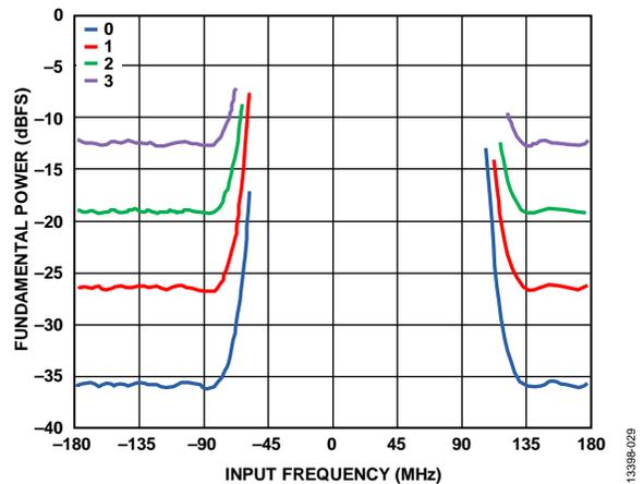
Figure 29. Frequency Sweep in VDR Complex Mode with Wideband Mask
