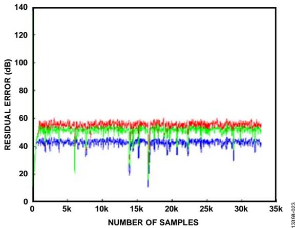
Figure 23. Residual Error for 9-Bit to 14-Bit Resolutions
