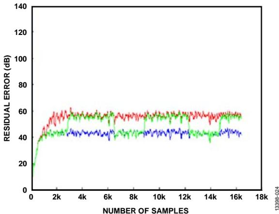
Figure 24. Residual Error with High and Low Resolution with VDR
