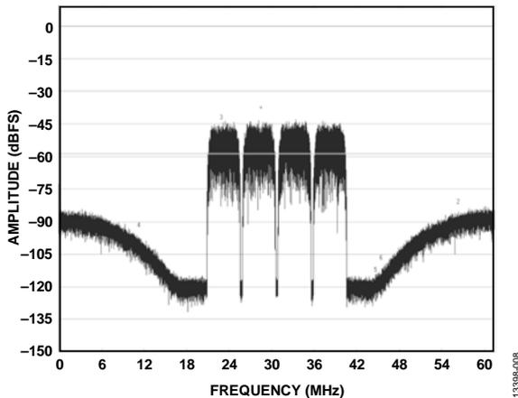
Figure 8. Noise Shaping in an FFT
