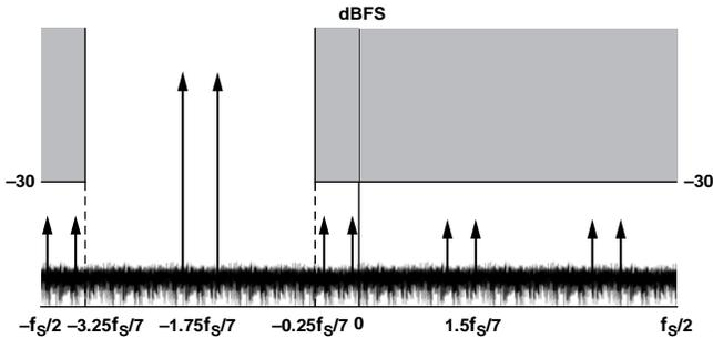
Figure 19. Complex Mode VDR Tuned for Negative Frequencies
