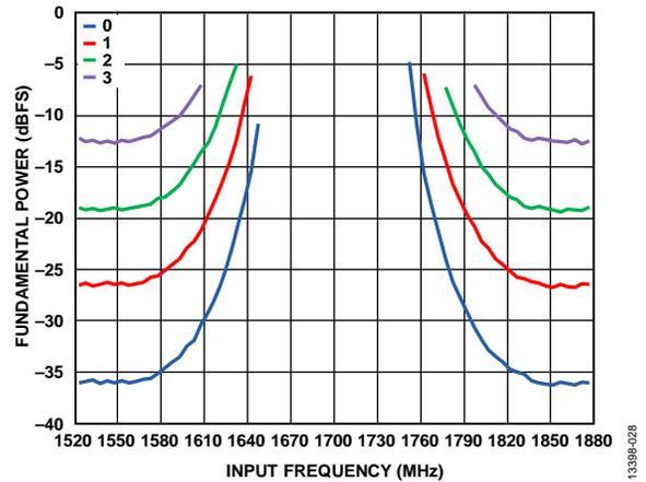
Figure 28. Frequency Sweep in VDR Complex Mode with Narrow-Band Mask
