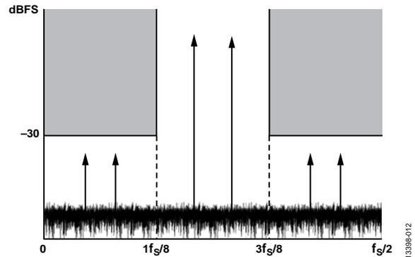
Figure 12. Simplified Diagram of VDR Frequency Bands
