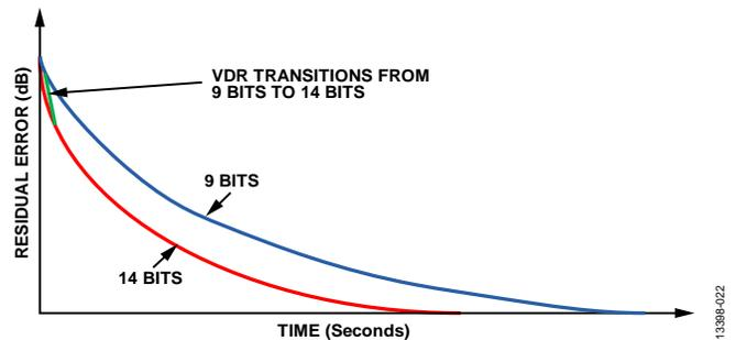
Figure 22. Residual Error vs. Time for 9-Bit and 14-Bit Resolutions
